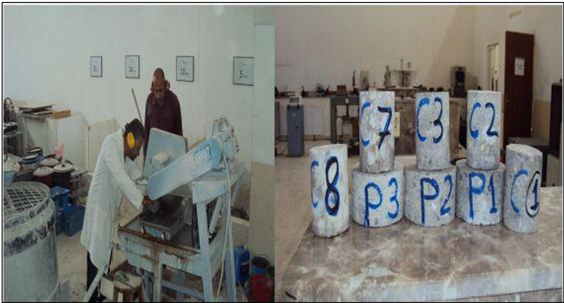
Figure 5.4: Sampled Core Cutting Process for Test.
