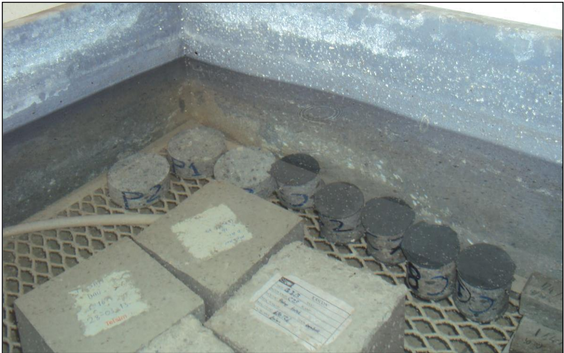
Figure 5.6: Curing Process of Specimens
