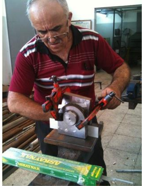
Figure 3-34: a) Hole making for pin connections .b) Adjusting pin connection pieces
