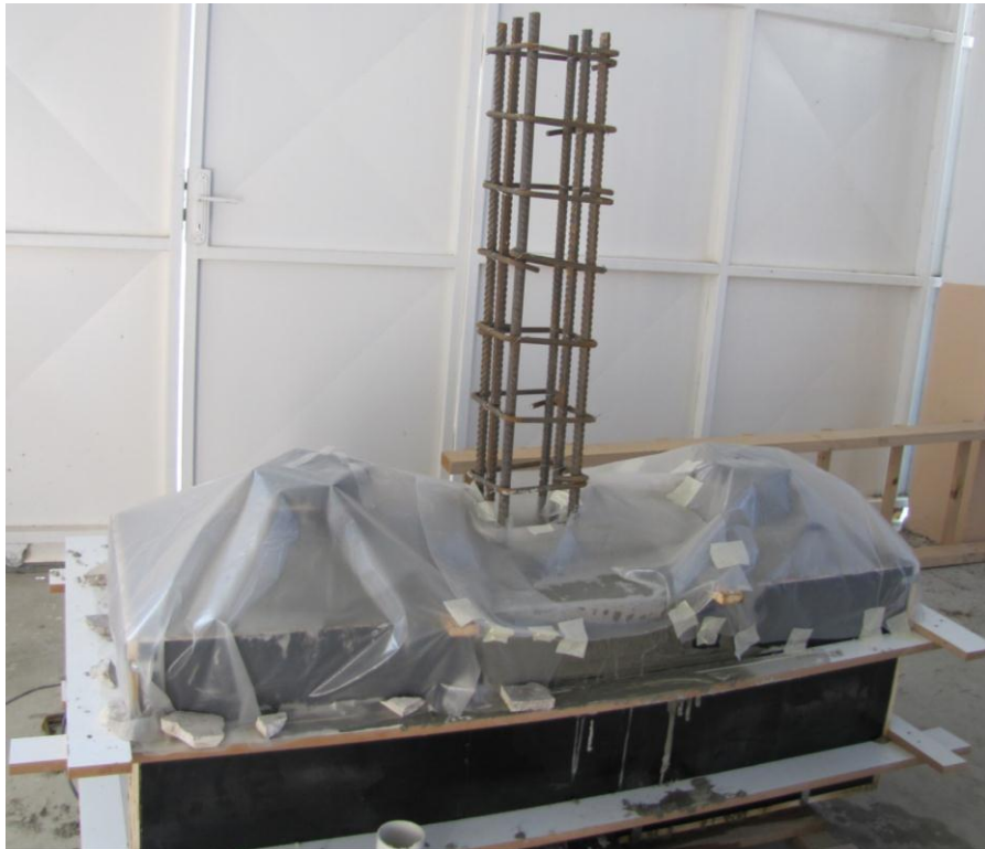
Figure 3-28: Covering the concrete surface
