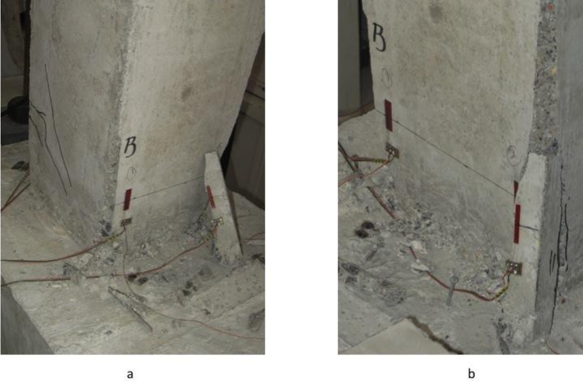
Figure 4-9: Start of crushing in compression side of the column without fibers
