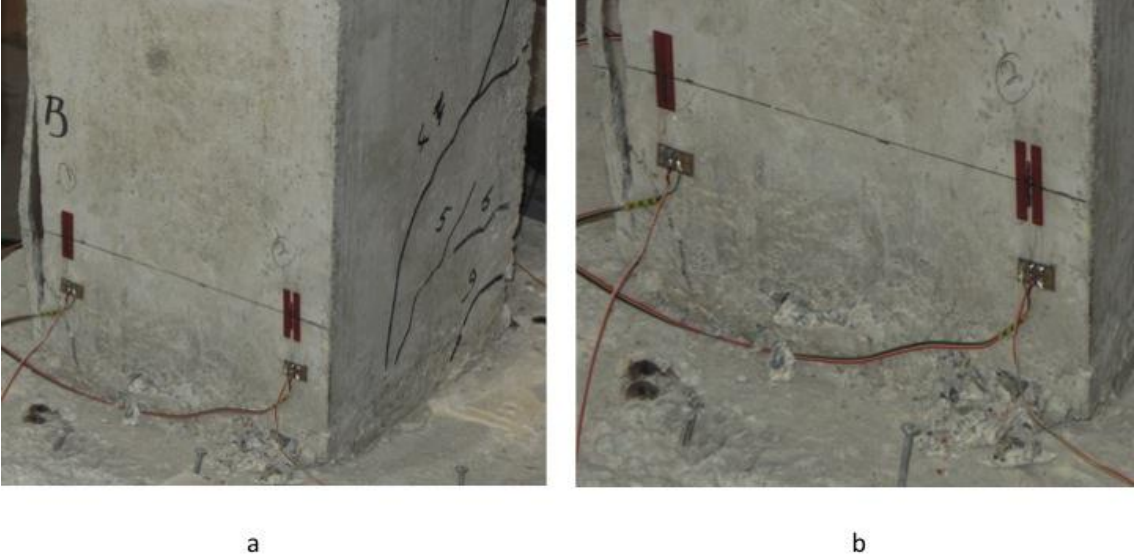
Figure 4-9: Start of crushing in compression side of the column without fibers
