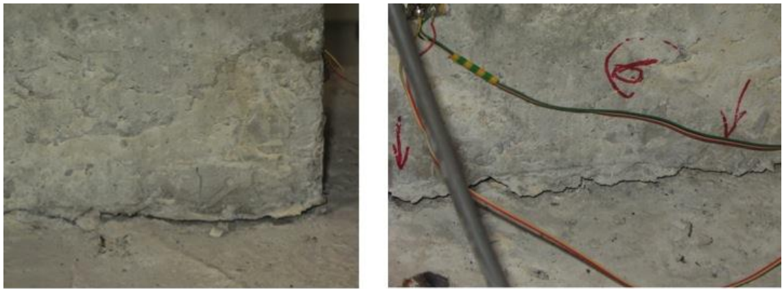
Figure 4-2: Slip in footing-column joint of column without fibers
