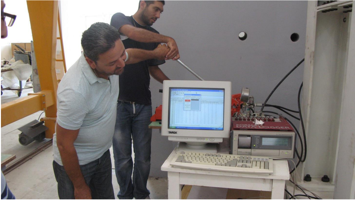
Figure 3-40: Applying loads manually and recording data with data logger
