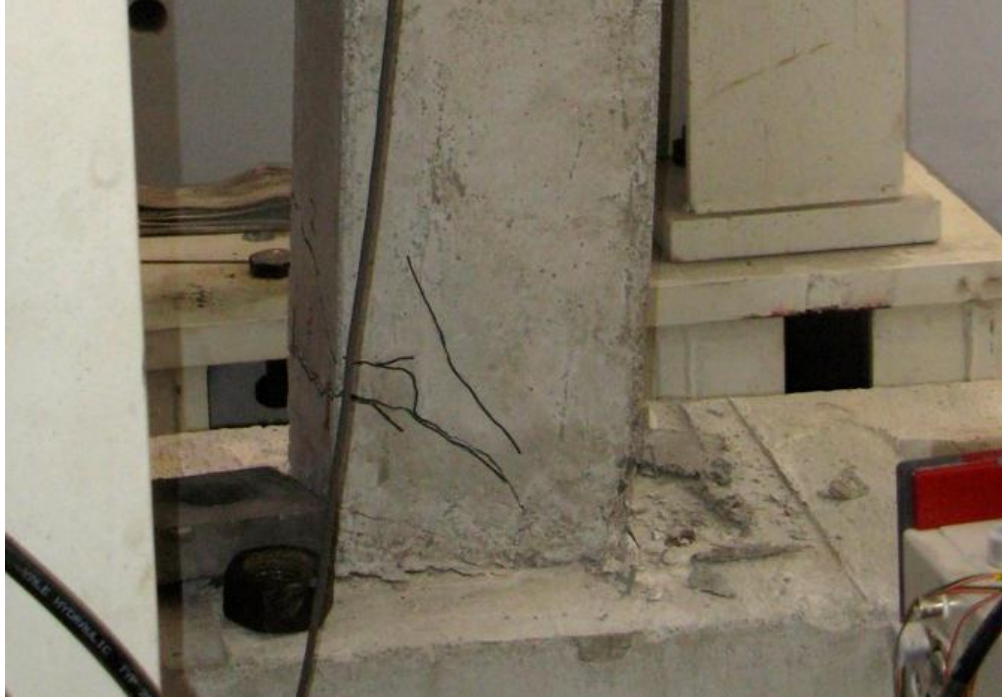
Figure 4-2: Slip in footing-column joint of column without fibers
