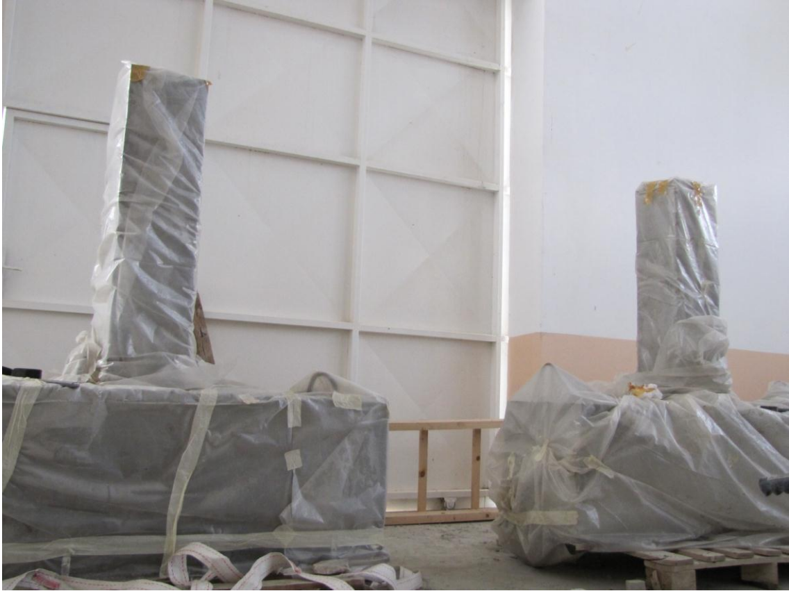
Figure 3-29: Curing the specimens
