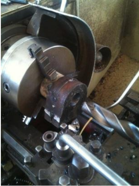
Figure 3-34: a) Hole making for pin connections .b) Adjusting pin connection pieces
