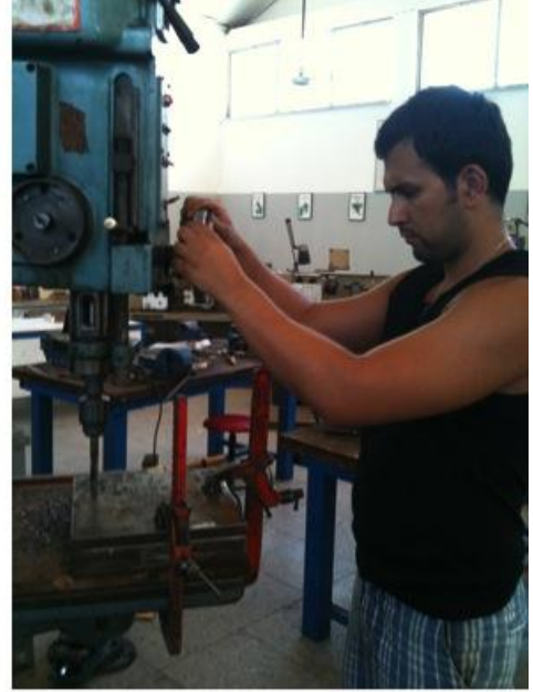
Figure 3-33: a) Making holes in the main steel base plate .b) Making holes in other steel plates
