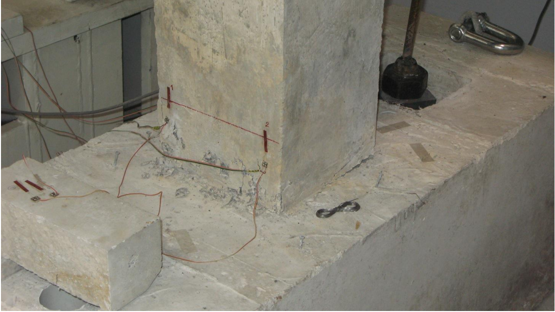
Figure 4-17: Crushing of the column with 1.5% fibers
