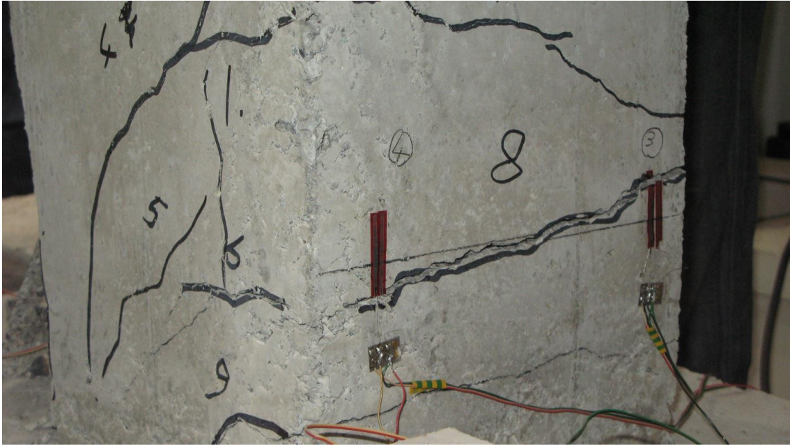
Figure 4-7: Ultimate cracks in tension side of the column without fibers
