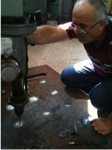
Figure 3-33: a) Making holes in the main steel base plate .b) Making holes in other steel plates
