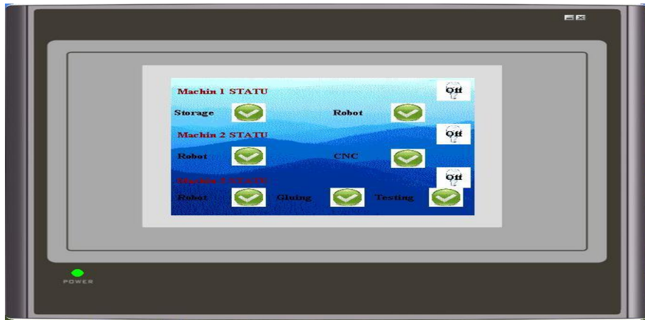
Figure 31:HMI Monitoring System
