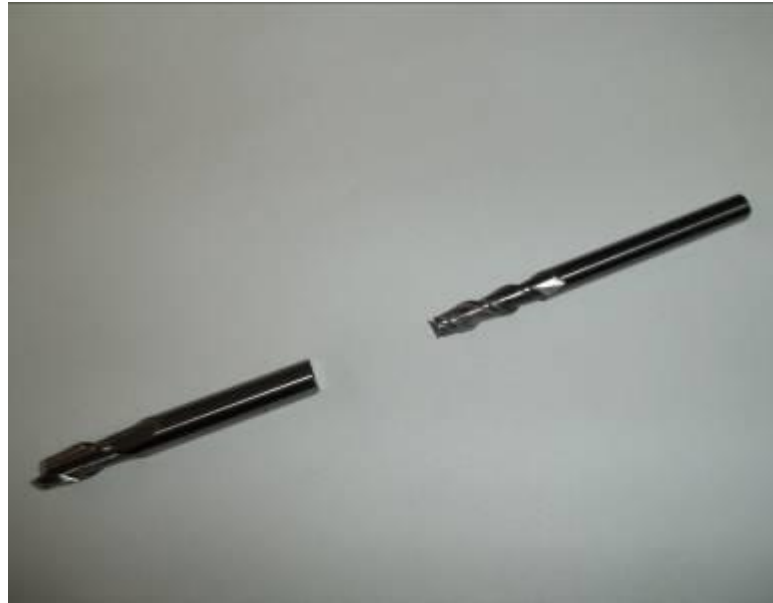
Figure 16: Twist drill (left) and end mill (right) used in the experiments.
