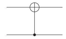
Figure 1.1: Controlled-Not Gate
