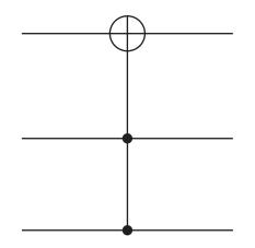
Figure 1.2: Controlled-Controlled-Not Gate (Toffoli Gate)
