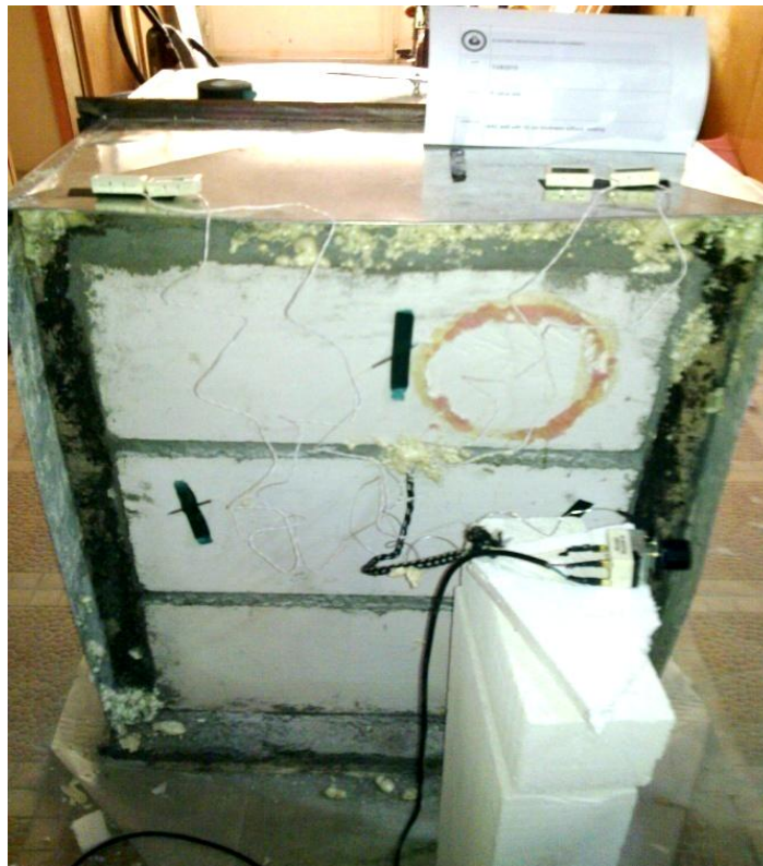
Figure 3.12: Thermal conductivity test setup
