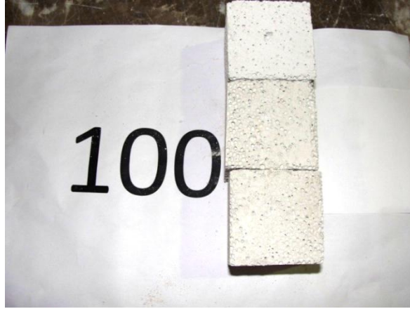
Figure 4.20: AAC blocks after heating at 100 °C
