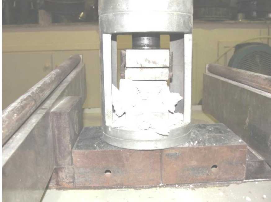
Figure 4.26: AAC sample after exposing 1000°C under compressive load
