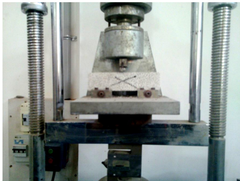
Figure 3.5: Flexural strength test apparatus.
