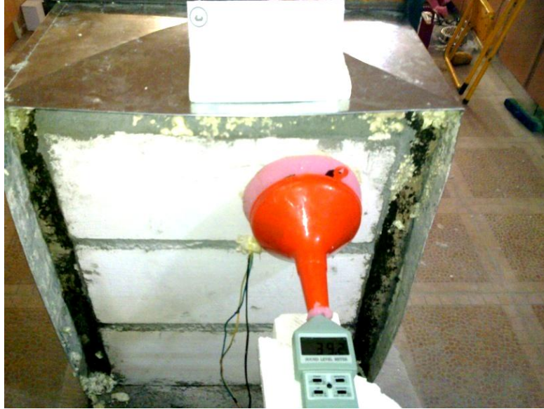
Figure 3.8: Sound level measuring test process
