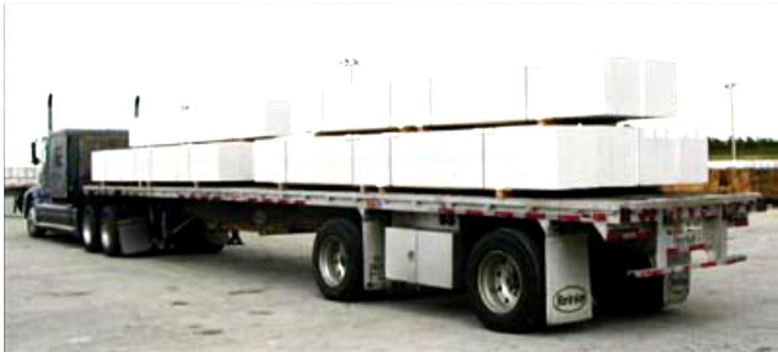
Figure 2.5: Transportation of the AAC to jobsite [1]
