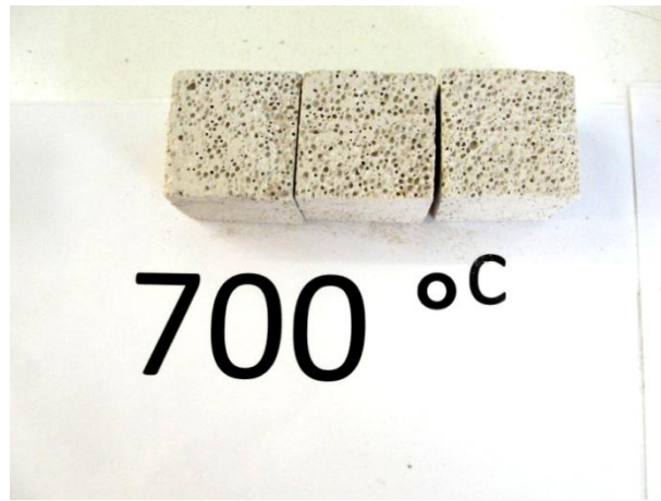
Figure 4.23: AAC blocks after heating at 700°C
