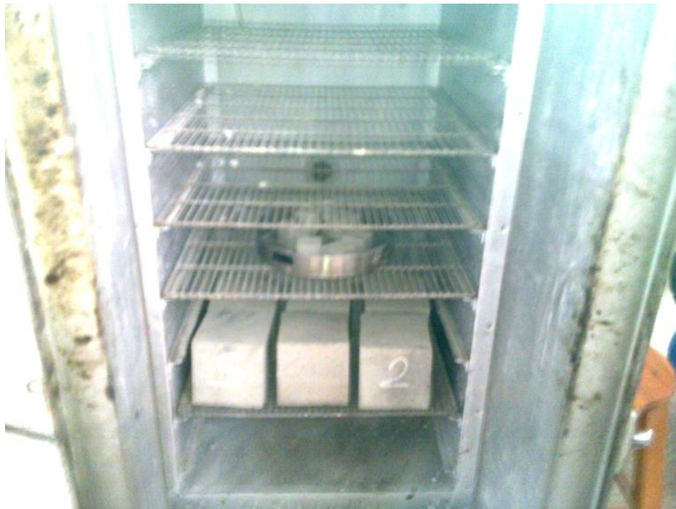
Figure 3.2: Specimens in oven for drying process.
