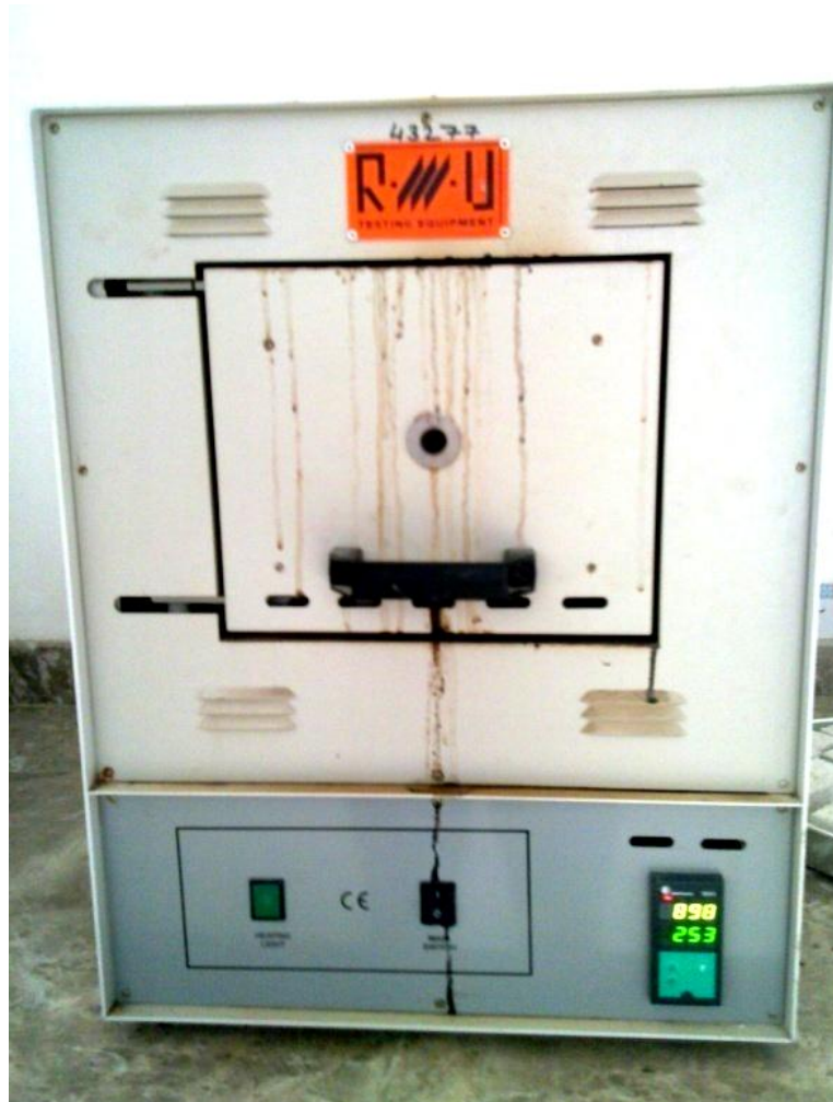
Figure 3.9: Fire resistance test apparatus
