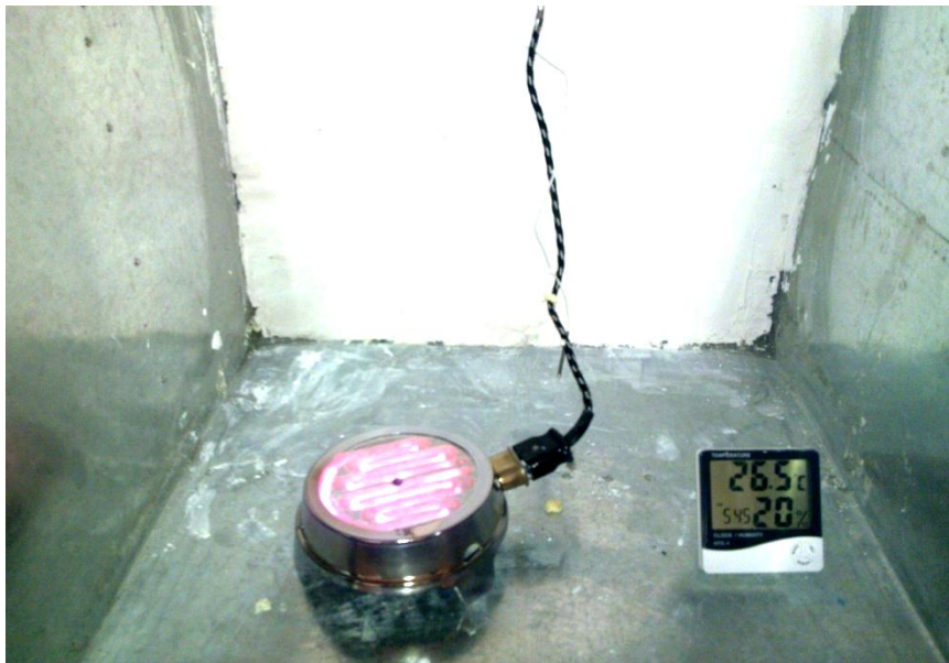
Figure 3.11: Heat production inside the chamber with electrical fire source.
