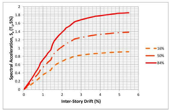
Figure 5.4. The summary of IDA curves for 6-story building (Near fault ground motions).
