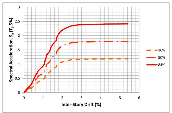
Figure 5.2. The summary of IDA curves for 6-story building (Far fault ground motions).
