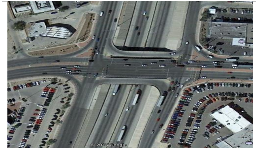
Figure 2-6: Diamond interchange U turns exclusive N-Lee Trevino Dr. interchange in El Paso-Texas-USA [14]
