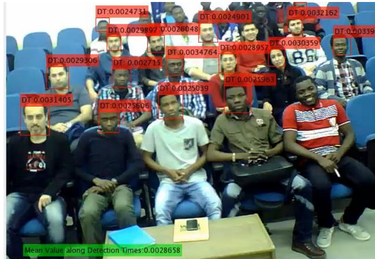
Figure 18: The Result of Implemented Method for Detection and Tracking for more than 30 People
