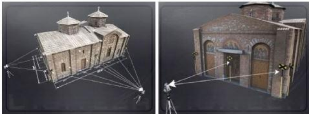
Figure 47: 2D or 3D measurements by one or two photos, (Tsioukas, 2003)
