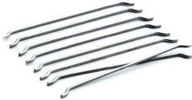
Figure 1: Hooked-end steel fibers (Lachemi et al. 2013)
