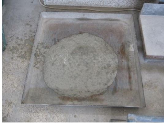
Figure 28: Slump and T50 tests
