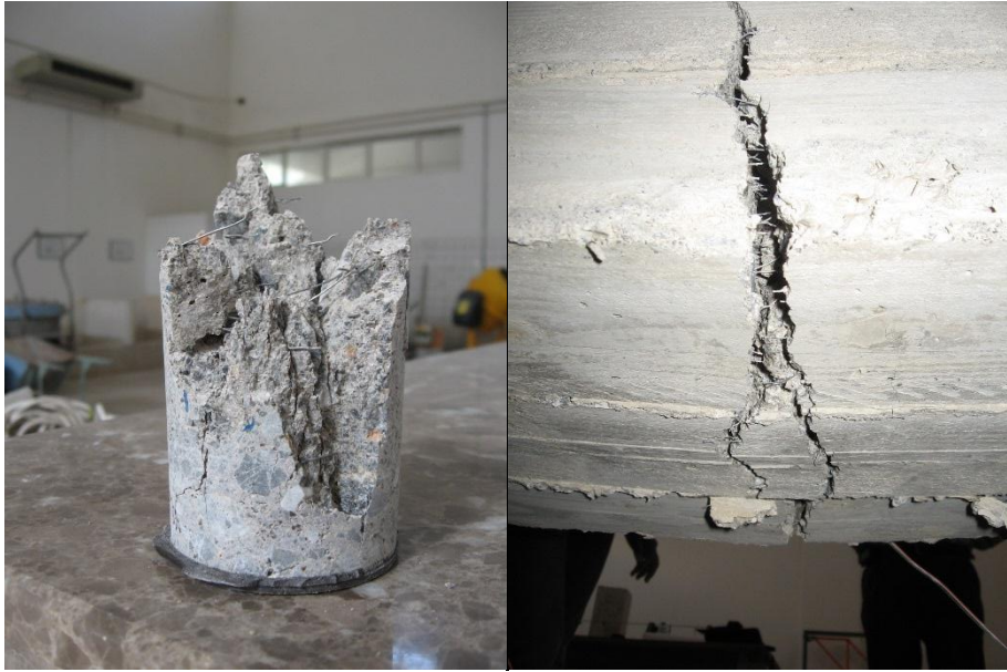
Figure 67: Fibers for bridging cracks
