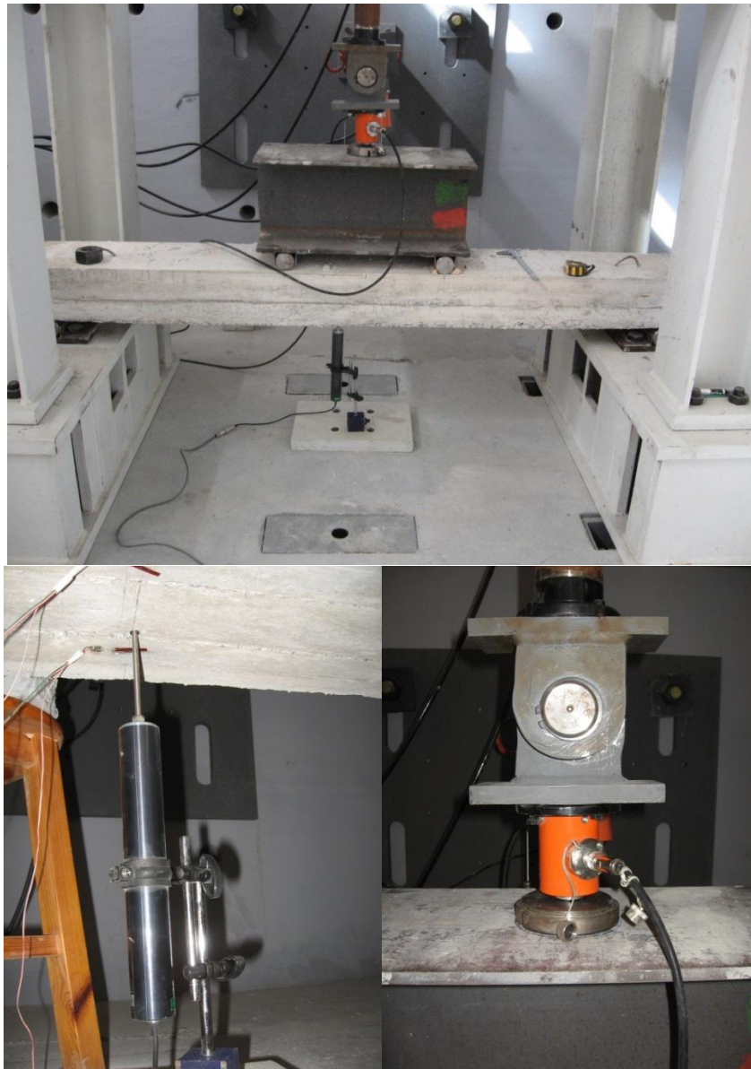
Figure 35: Test apparatus for flexural strength
