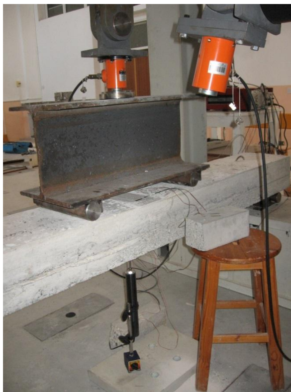
Figure 37: Test apparatus (load cell, IPE400 and transducer)
