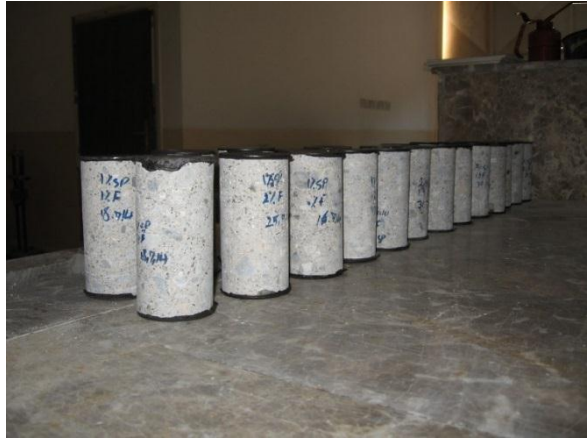
Figure 64: Core sample for Stress-Strain curvature
