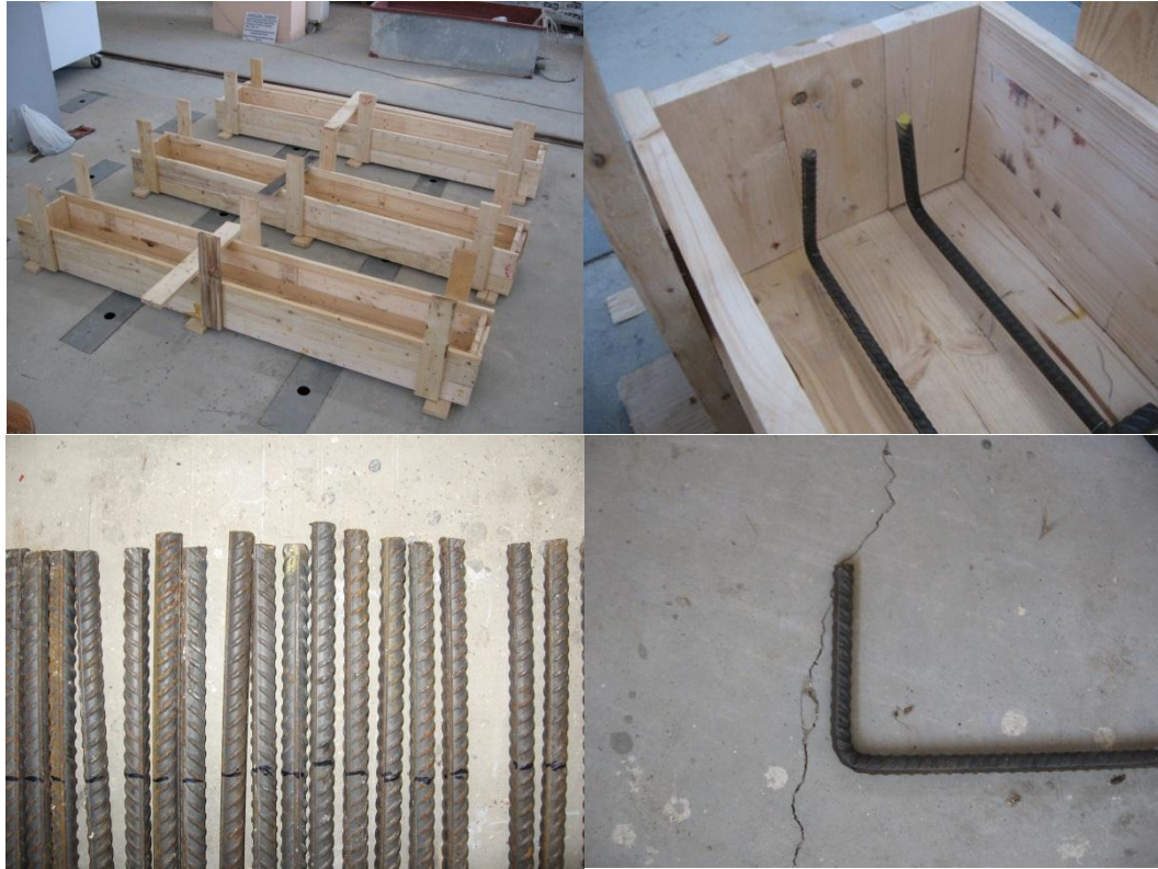
Figure 24: Formwork construction and bars
