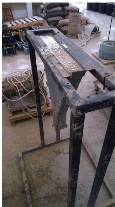
Figure 32: V funnel test
