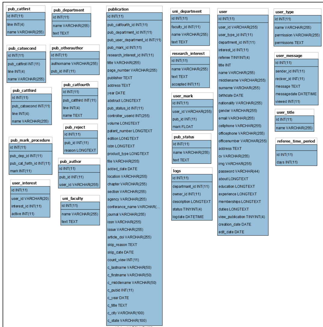
Figure 2.16: Class Diagram of the System
