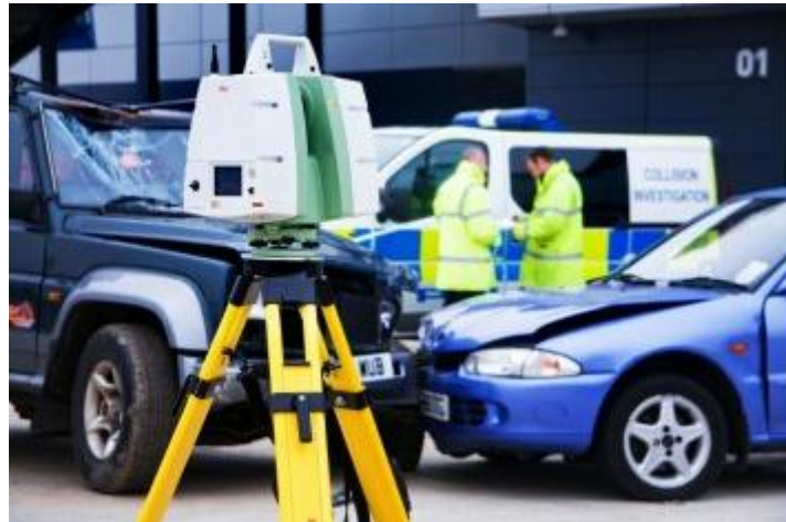
Figure 27: Laser Scanning in Accident Investigation
