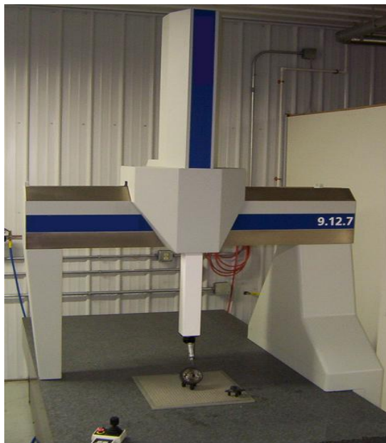
Figure 16: Contact Laser Scanning (coordinate measuring machines with rigid perpendicular arms)
