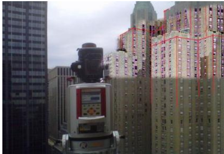
Figure 24: Laser scanning for surveying
