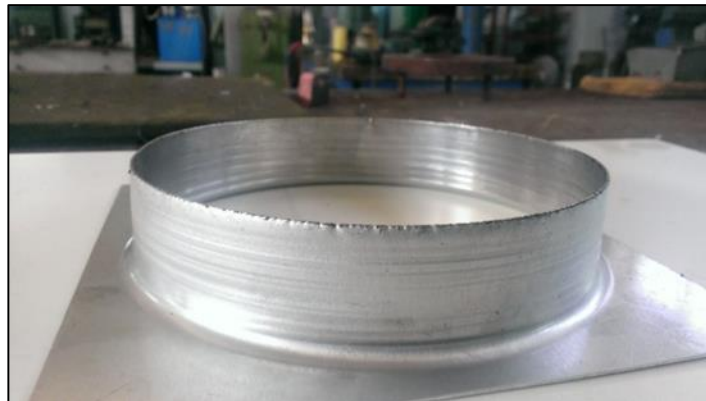
Figure 5.5: 90 mm holed part – No failure occurred.
