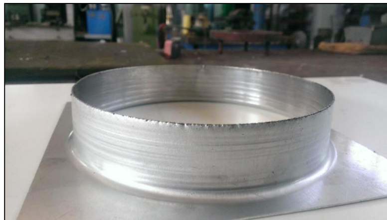
Figure 5.2: 95 mm holed part – No failure occurred.
