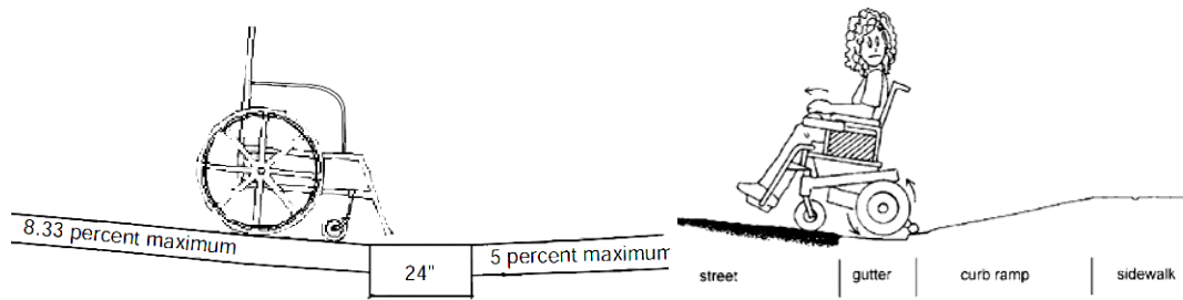
Figure 3.17: Provide 24 Inches between Close Interval Grades (Kirschbaum, et al., 2001, p.7-32)
