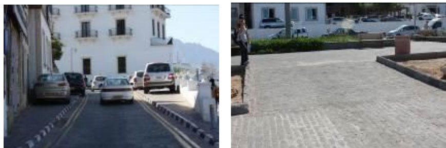
Figure 4.33: Rapid Changes in Gradient Cause Upward Movement Difficult
