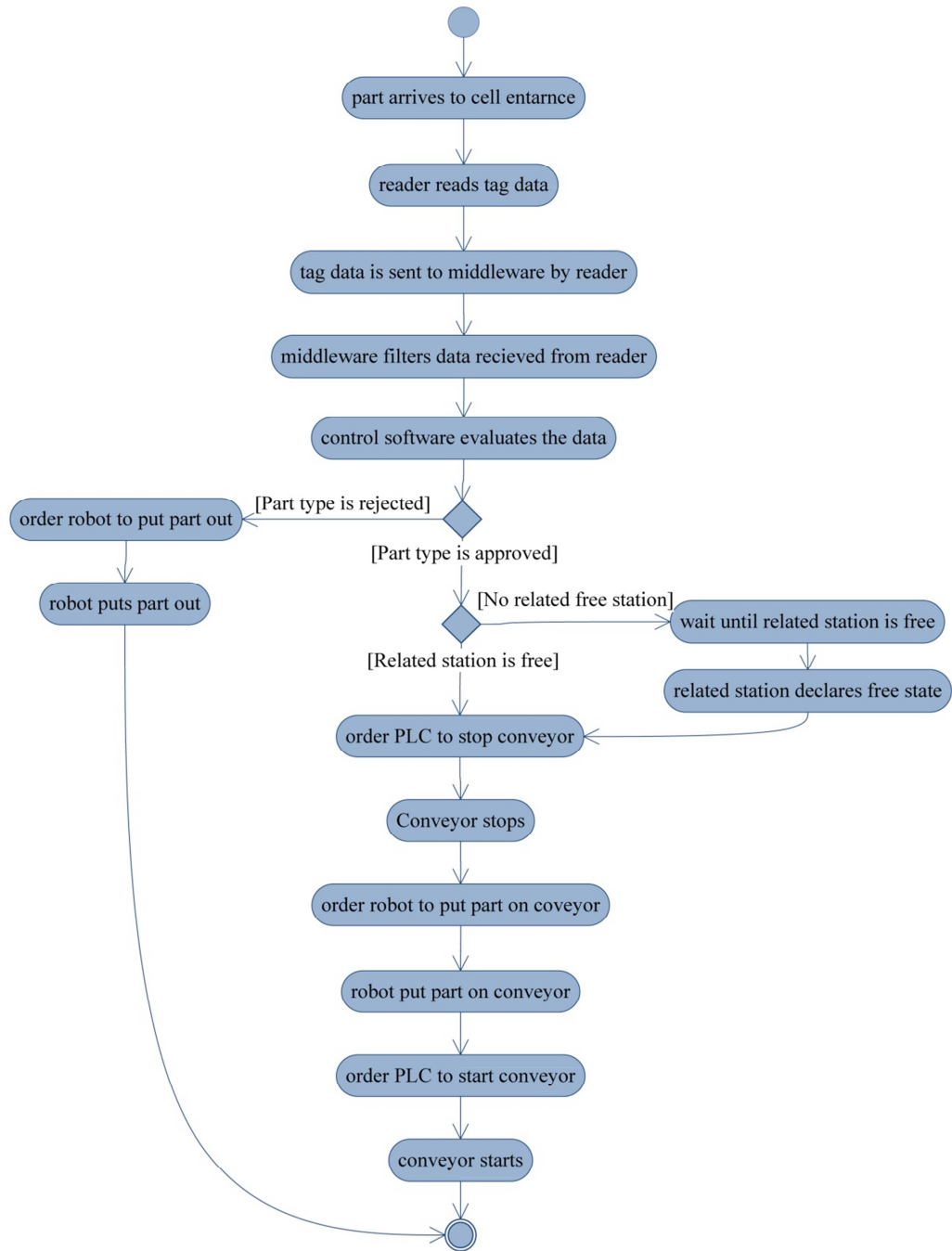
Figure 3.3: Process of Entering Part to Cell
