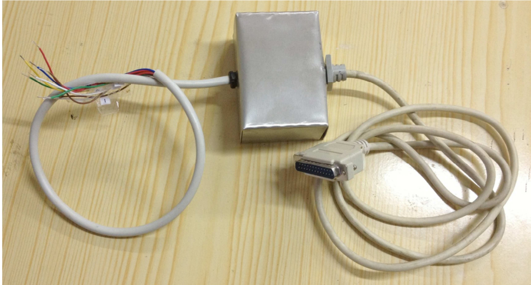
Figure 4.7: PC to PLC Hardware Interface
