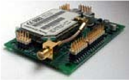
Figure 5: A PC104 single board computer running on Linux used to produce the terminal device.
