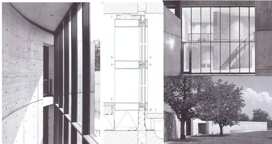
Picture 23: Facade Detail of Typical Aluminium Profile for Glass Curtain Wall System at the Conference Pavilion Building and a Detail Section of the Curtain Wall (Schittich, C. et al, 1999).
