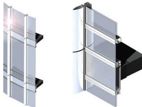
Figure 35: Anchored Floor Slab to Glass Panel and 3 Dimensional Images for Burj Tower (Peter. A. W, Gregory L. S, Mohamed. S, Skidmore, Owings and Merrill. 2007)
