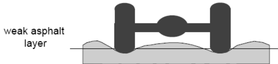
Figure 23: Deformation of the flexible pavement due to poor HMA design (Druta, 2006, p. 117)
