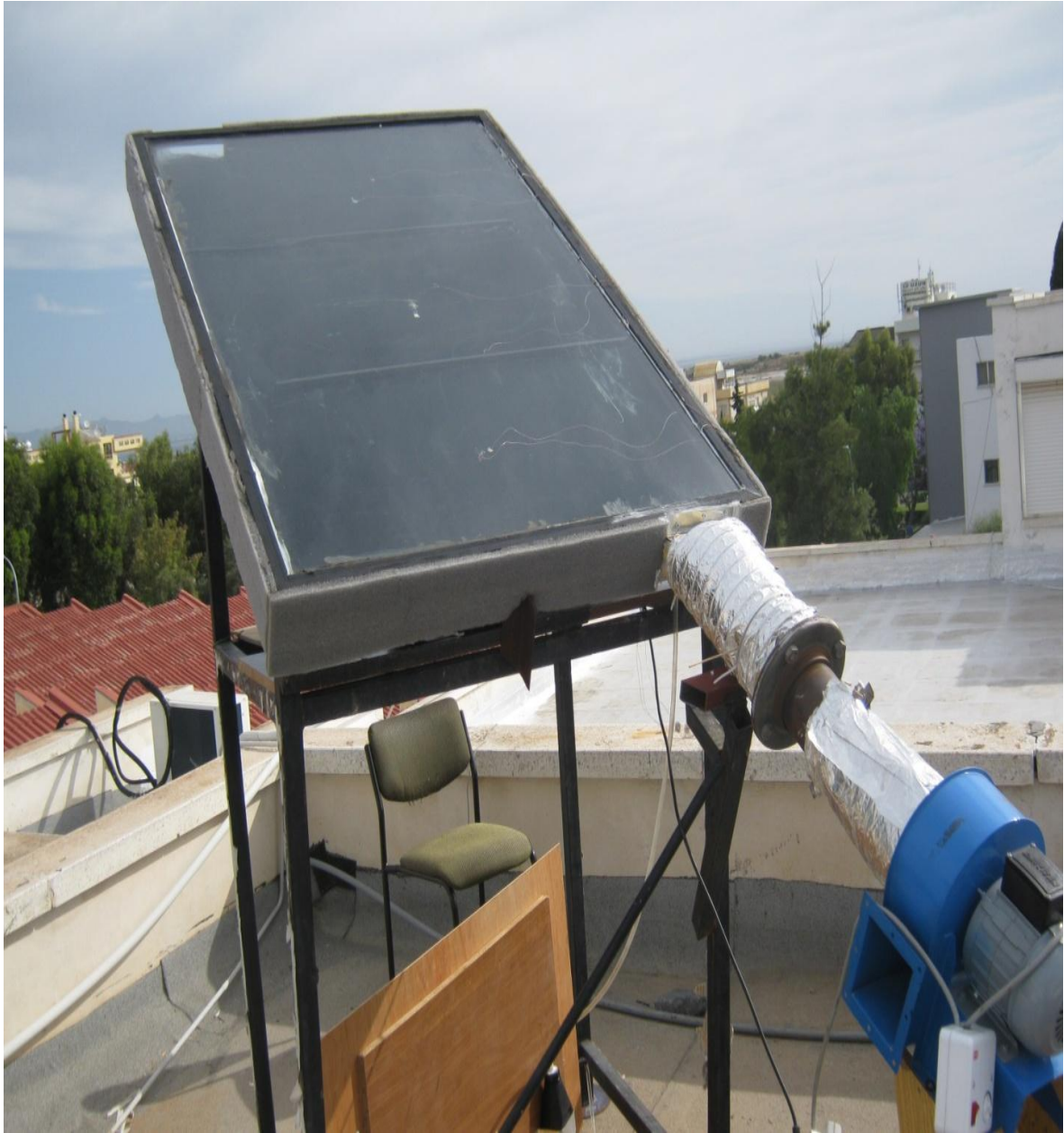
Figure 2.3: Pictorial view of the experimental set up for SPSAHWR .
