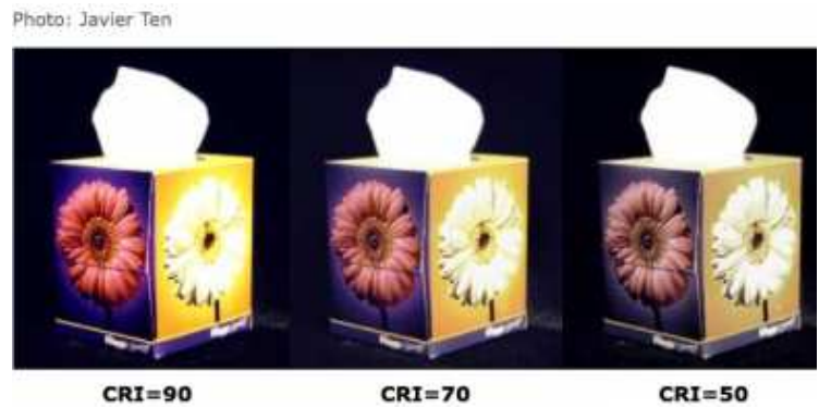
Figure 25. An object illuminated with light sources of different CRI values (URL 12: Goldberg, 2010) www.techbites.com
