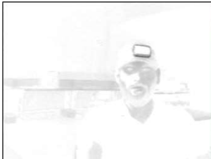
Figure 8. The Negative Normalized Red Component after Median Filter.
