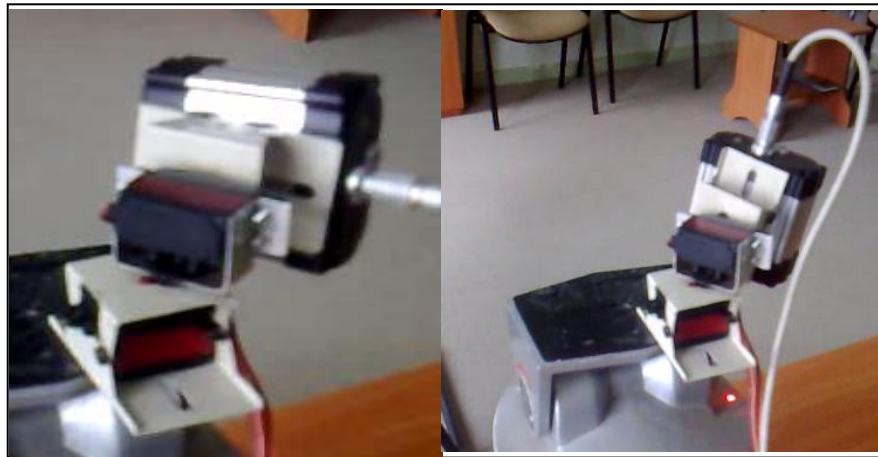
Figure 2.11: 3-D laser scanner by using a 1-D range finder and a servo motor-based Pan-tilt
