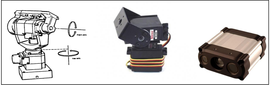
Figure 2.8: (a) Servo motor based Pan-tilt's rotation principle, (b) servo motor based Pan-tilt, (c) 1D Lidar (Noptel CMP3-30,) [35], [26].
