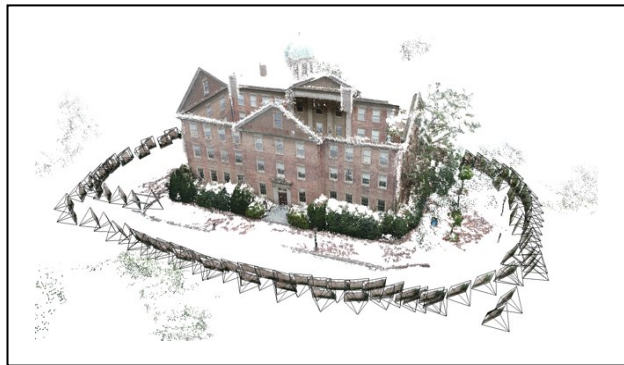
Figure 1.4: Taking scan from different angels, [15].
