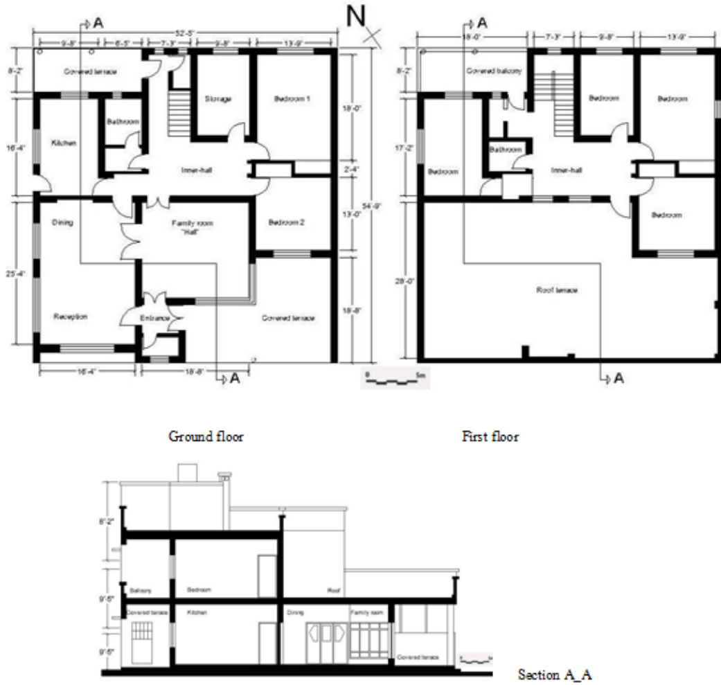
Figure 125: Ground and first floor plan and section of Mandilawi house in Baghdad (Mandilawi, 2012)
