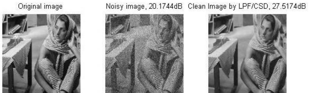
Figure 10: Denoising using LPF/CSD algorithm. Algorithm parameter d=1 , \lambda = 1.8
