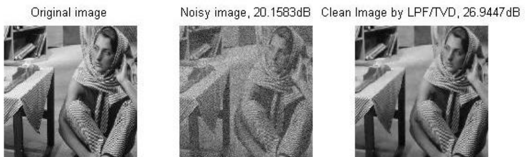
Figure 9: Denoising using LPF/TVD algorithm. Algorithm parameter d=1 , \lambda = 1.5
