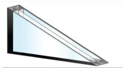
Figure 14: Cutaway of triple- pane insulated glass unit (Sharma, 2014)
