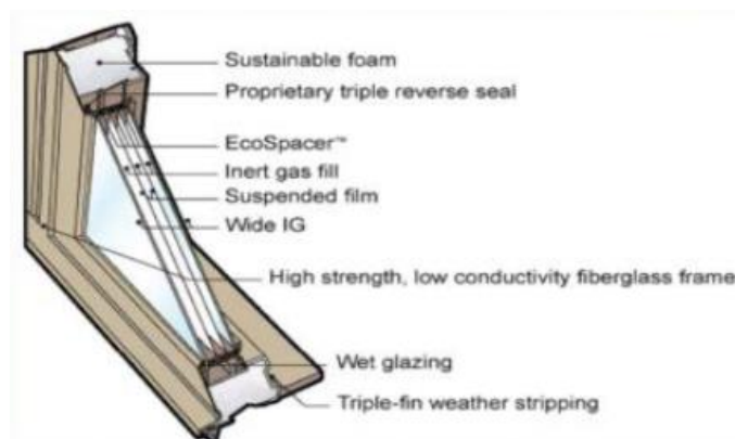
Figure 15: Cutaway of a quad pane window including the frame (Sharma, 2014)
