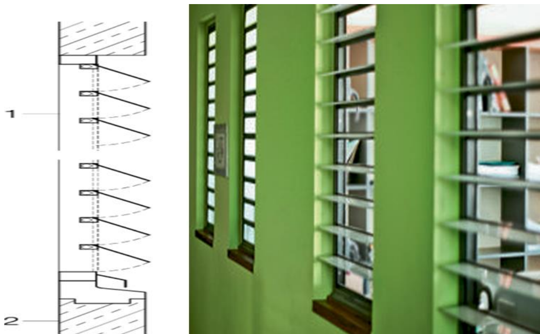
Figure 70: Section, wall with louvered windows, scale 1:20 (Voss et al., 2013)
