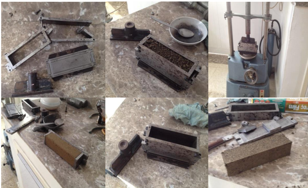
Figure 3.10: Special mold for preparing compacted soil beam and the equipment used for static compaction.
