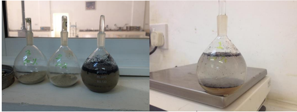
Figure 3.5: Determination of G_s of Soil- STR mixtures with rubber floating on the surface of water.
