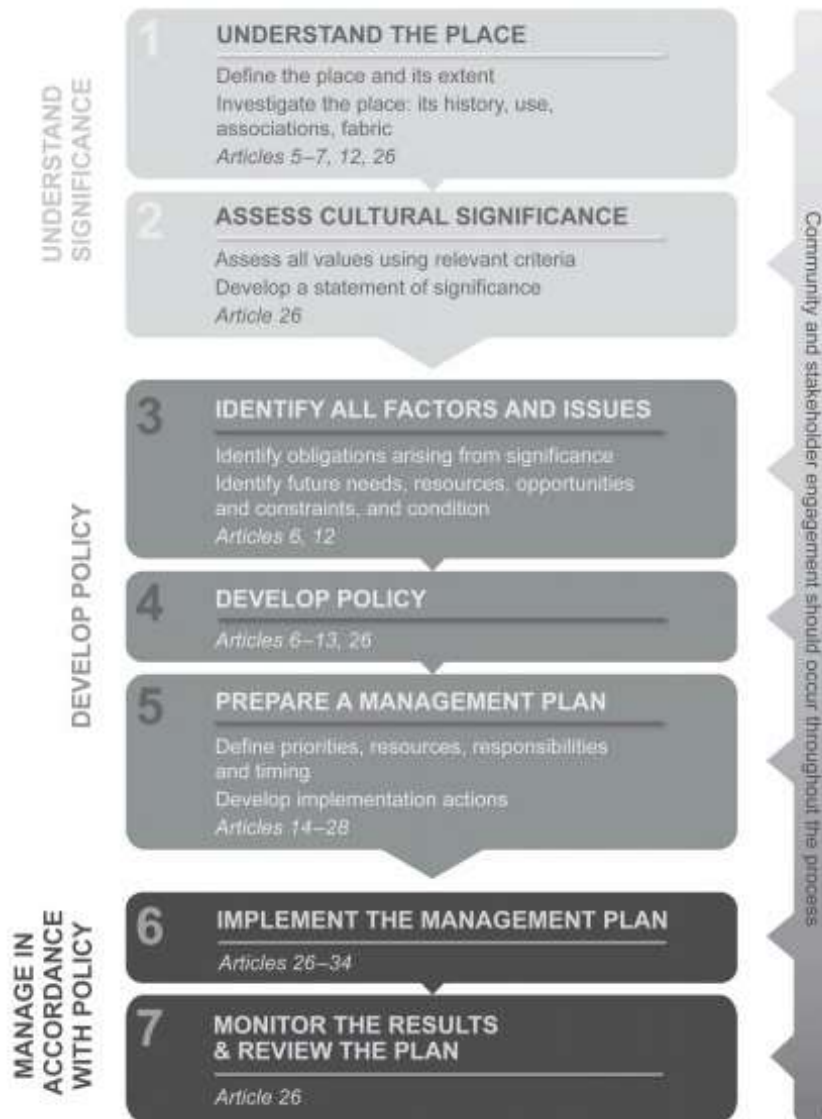
Figure 8. The Burra Charter Process. Steps in planning for and managing a place of cultural significance. Key articles relevant to each step are shown in the boxes. (URL3)
