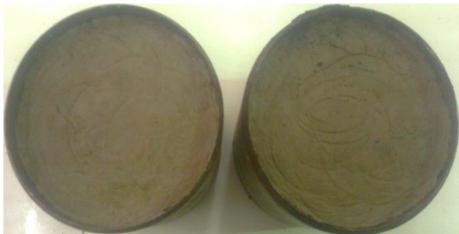
Figure 3.3: The compacted clay soil in the molds
