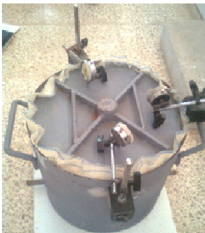
Figure 3.20: The complete set up with deformation gauges
