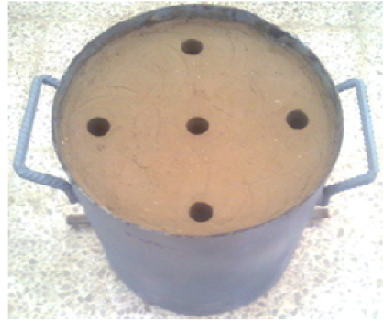
Figure 3.15: The columns of 3 cm in diameter constructed with PVC pipe in the clay sample block
