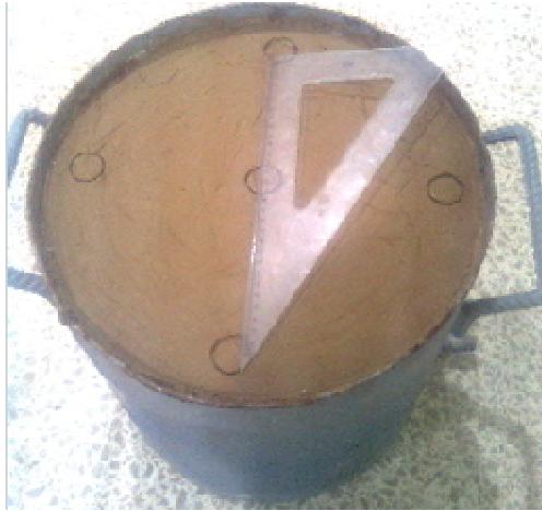
Figure 3.14: The position of the four columns marked at 18 cm to each other and 12 cm to the central column
