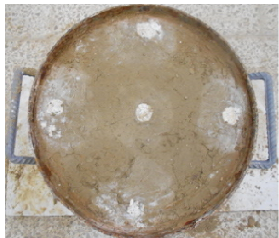
Figure 3.21: The treated soil after 90 days of curing with quicklime
