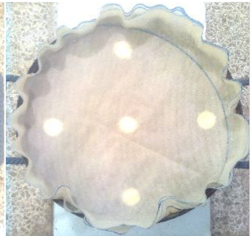
Figure 3.17: Showing the placement of the thin porous fiber cloth
