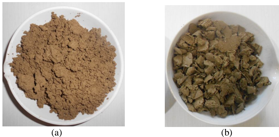
Figure 3.24: The textural appearance of the soil (a) Natural soil (b) Stabilized soil
