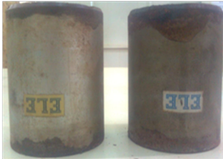
Figure 3.2: The steel molds used for preliminary setup
