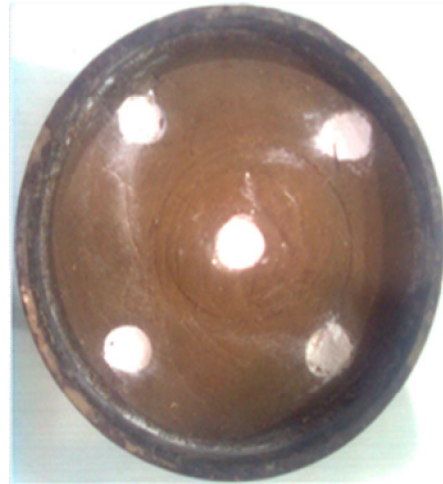
Figure 3.10: Picture showing the lime pile installation
