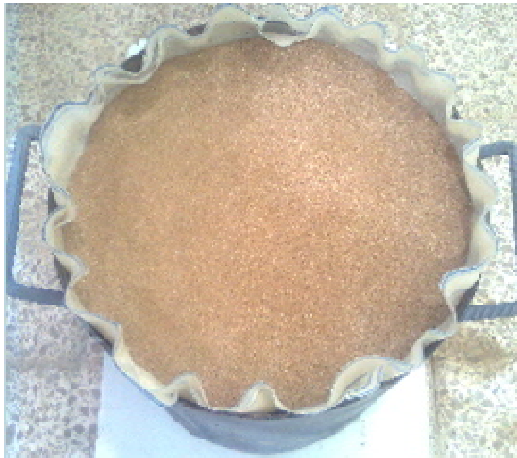
Figure 3.18: Showing the layer of sand soil on the porous fibre cloth
