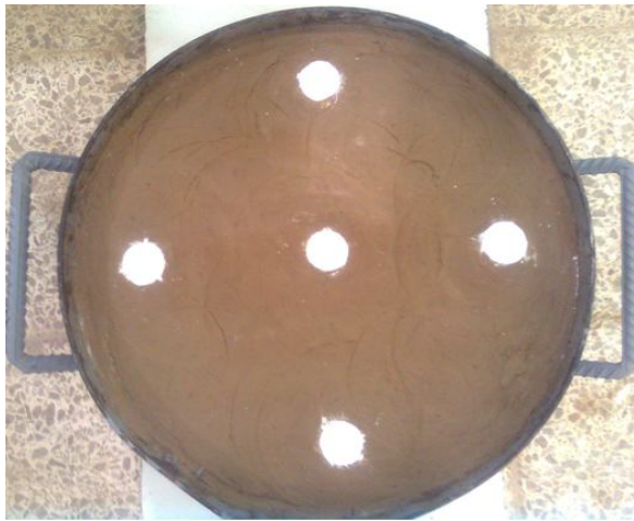
Figure 3.16: Pattern of the lime-piles installation in the soil block
