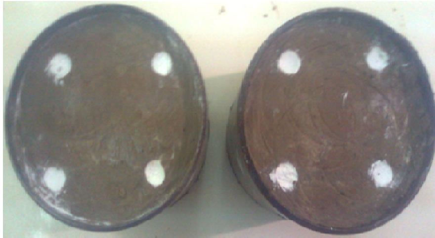
Figure 3.5: Pictures showing the lime-piles installation
