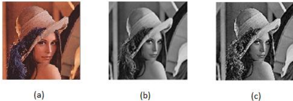
Figure 4-1.(a) Original Input Image; (b) Gray-Scale Image; (c) Preprocessed Image
