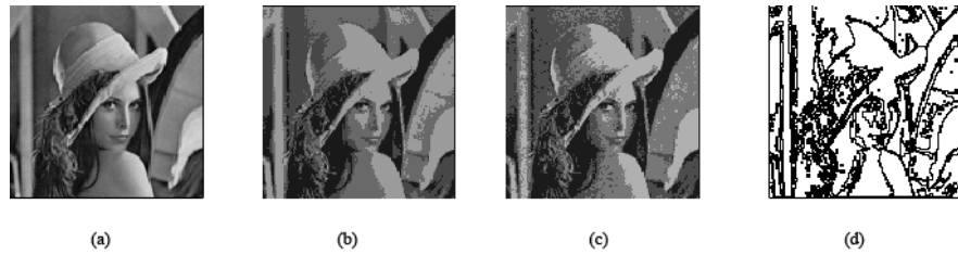
Figure 5-2. Test Image: (a) Corrupted Image with Gaussian Noise (Variance= 0.001 and Mean= 0.0); (B) Clustered Image Using K-Means Algorithm; (C) Separating Image by Drawing Boundary; (D) Region Detection
