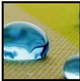
Figure 20. Liquid on Nano-Tex treated fabric (Sylvia Leydecker, 2008)
