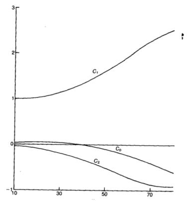
Figure 45. The original C constants for different  $\beta$  values (x Axis) plots from JRC Hsu and Evans (1989)
