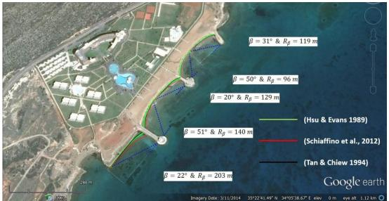
Figure 32. Application of the PBSE and its alternative modifications for unsubmerged headland tips at Noah's Ark Hotel embayment.
