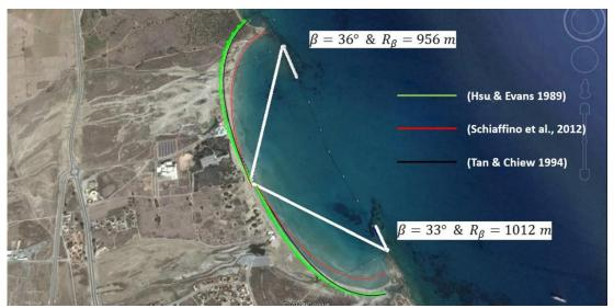
Figure 27. First application of the PBSE and its alternative modifications for unsubmerged headland tips to Kanlidere stream`s delta
