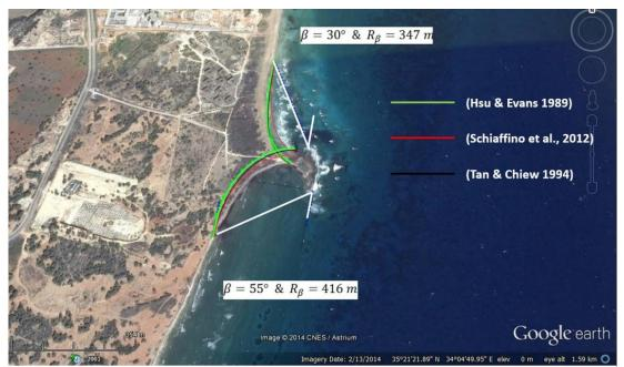
Figure 30. First application of the PBSE and its alternative modifications for unsubmerged headland tips at Artemis Hotel region.
