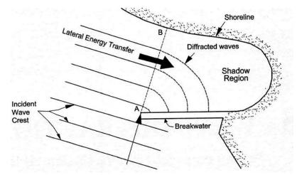
Figure 6. Schematic illustration of wave diffraction process
