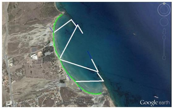
Figure 28. Multiple diffraction point used to fit the shoreline periphery of the beach by MEPBAY
