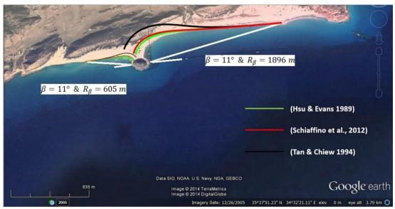
Figure 33. Application of three alternative PBSE modifications to the Golden beach embayment, picking the unsubmerged points on the headland as diffraction point
