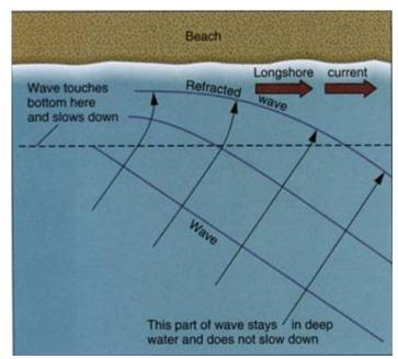
Figure 4. Wave Refraction and Longshore Currents (Plummer et al., 2001)
