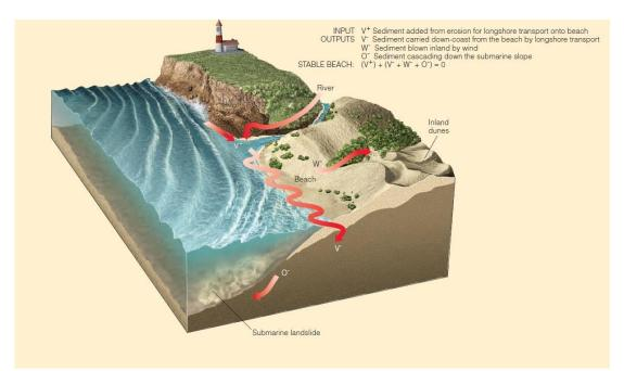
Figure 7. Nearshore sediment budget diagram (Monroe et al., 2006)
