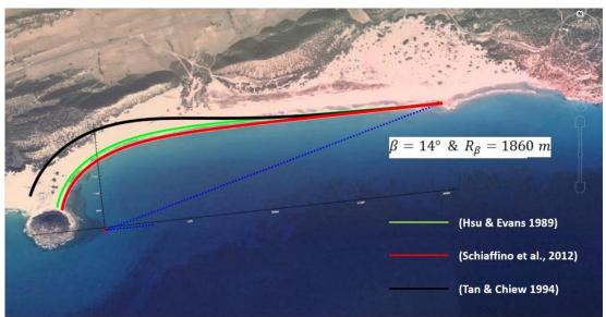
Figure 34. Result of choosing an alternative submerged diffraction point for the right headland of the Golden beach
