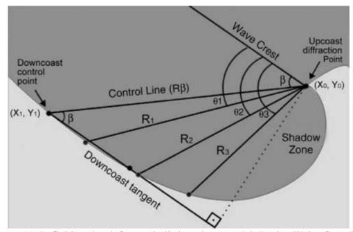
Figure 11. Definition sketch for parabolic bay shape model (Raabe, Klein, González, & Medina, 2010)
