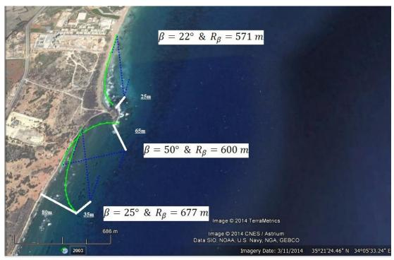
Figure 31. Length and direction of the headlands to reach the satisfactory diffraction point to reach an acceptable headland bay static equilibrium for Artemis Hotel area
