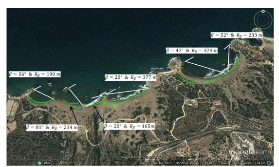
Figure 36. General implementation of the PBSE to different headland bays of the Alagadi Beach, using unsubmerged headland tips as diffraction points
