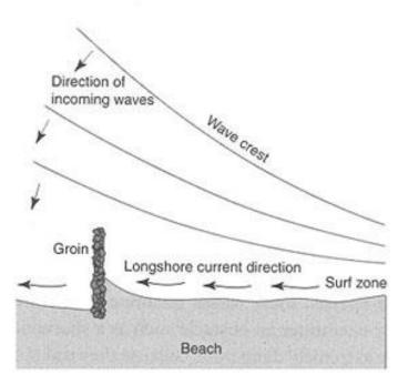
Figure 5. Sediment transportation as a result of longshore currents
