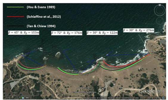
Figure 38. Implementation of different expressions of the PBSE on the west side bays of the Alagadi beach for more detail observation considering submerged diffraction points
