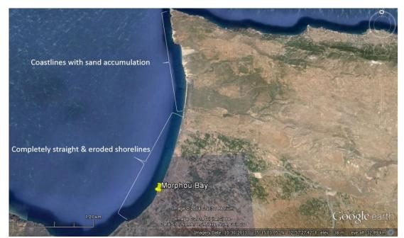
Figure 44. Sand accumulation location updrift of the Morphou bay
