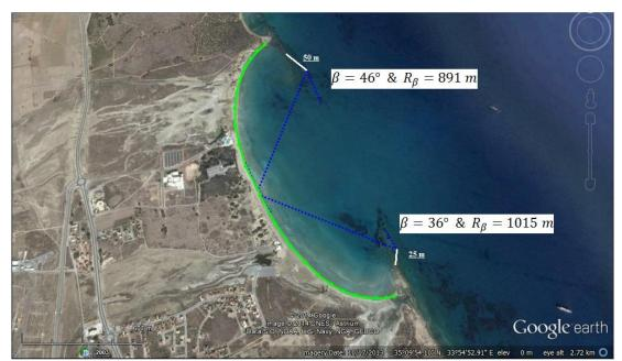
Figure 29. Length and direction of the headlands to reach the satisfactory diffraction point to reach the double curved headland bay static equilibrium
