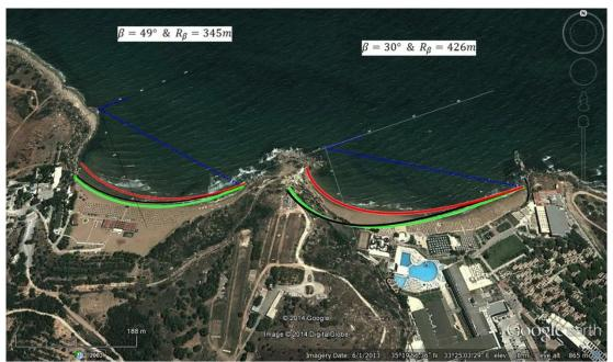
Figure 41. Unsubmerged diffraction points with right wave directions
