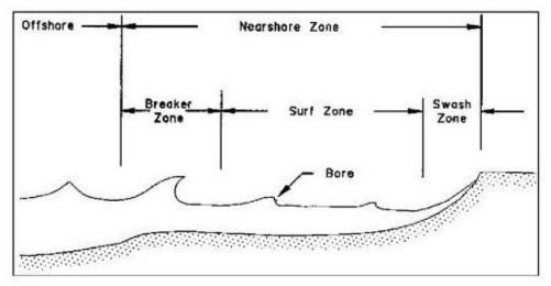
Figure 3. Nearshore wave processes terminology, (Leenknecht, 1992)
