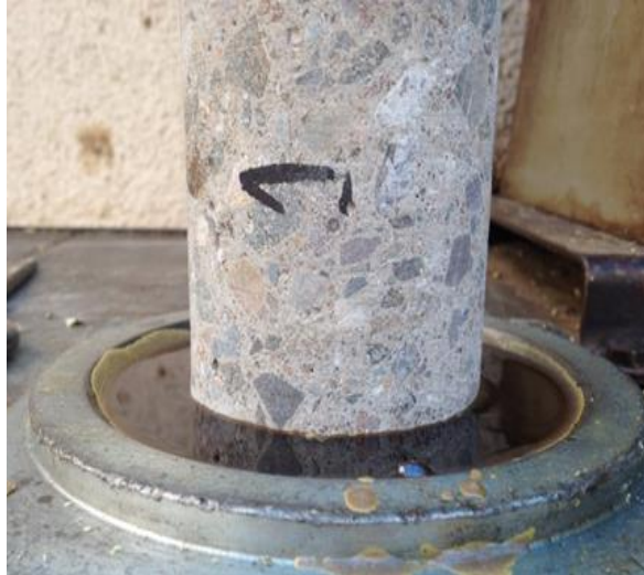
Figure 3.8. Capping of cylinder cores.
