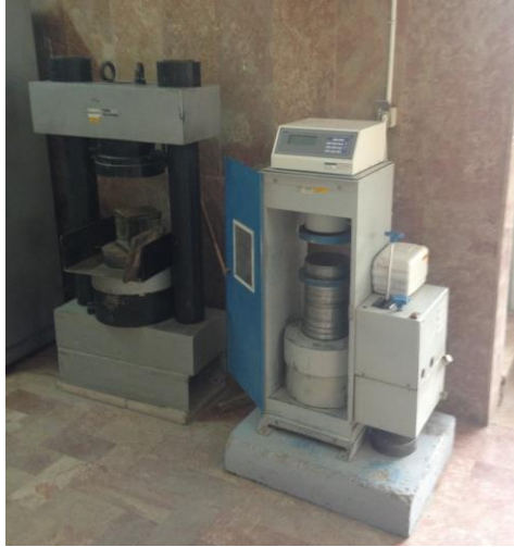
Figure 3.9. Compressive strength testing machine.
