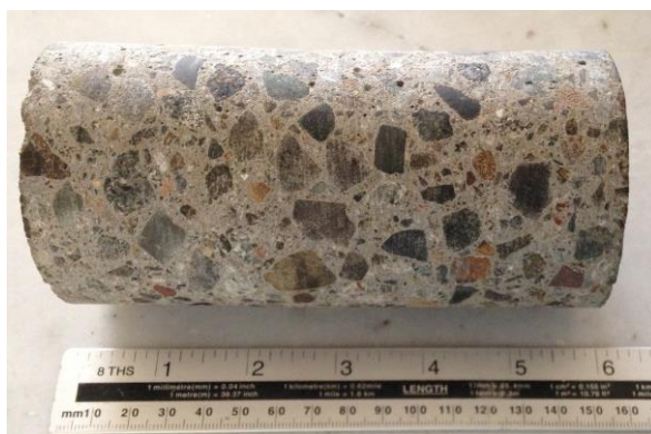
Figure 3.7. 7.5 cm concrete cylinder cores.
