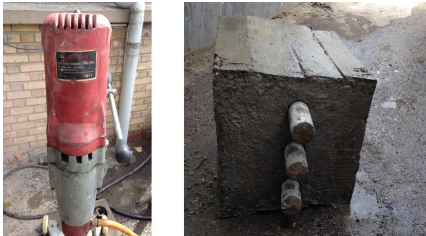
Figure 3.6. Drilling method of (50*50*50) cm specimens.
