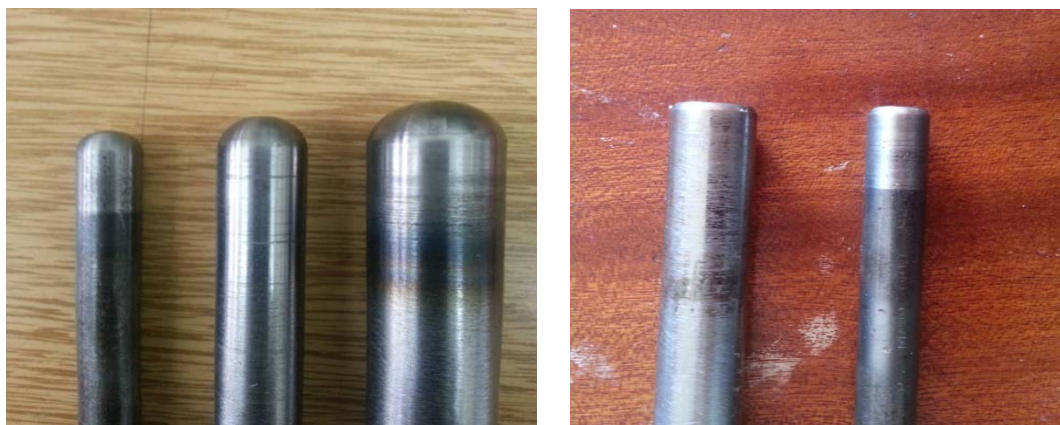
Figure 4.4: (A) Round end tools with diameters and 10,14 and 20mm. (B) Flat end tools with 10 and 14mm.
