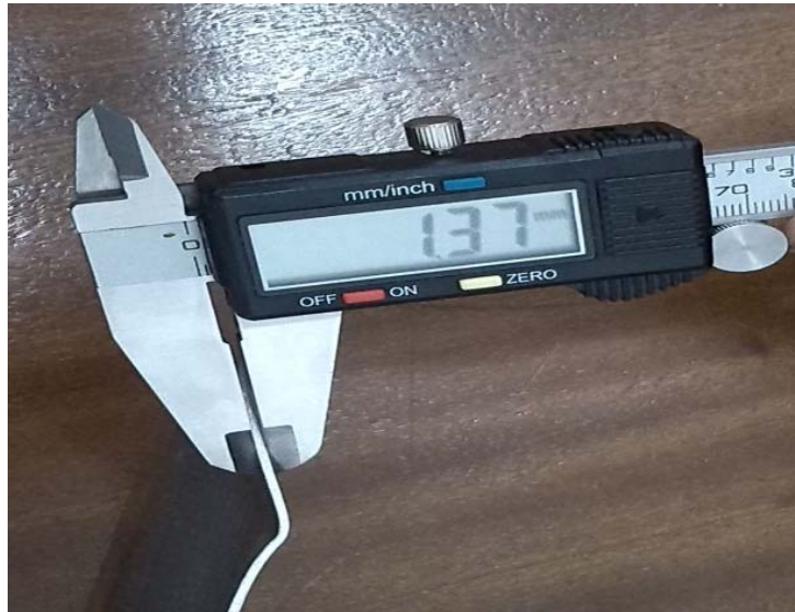
Figure 5.4: Measuring the variation in sheet thickness along profile of the sheet
