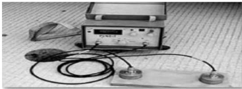
Figure 3.2: UPV Testing equipment (Proceq SA, 2013)
