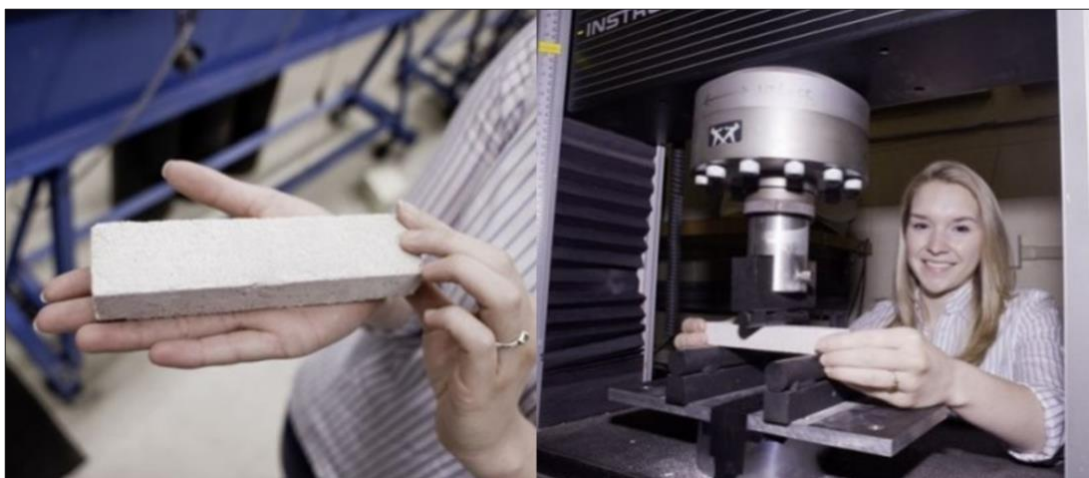
Figure 3.23: Self-healing concrete by Michelle Pelletier (2010), Source: (URL22)
