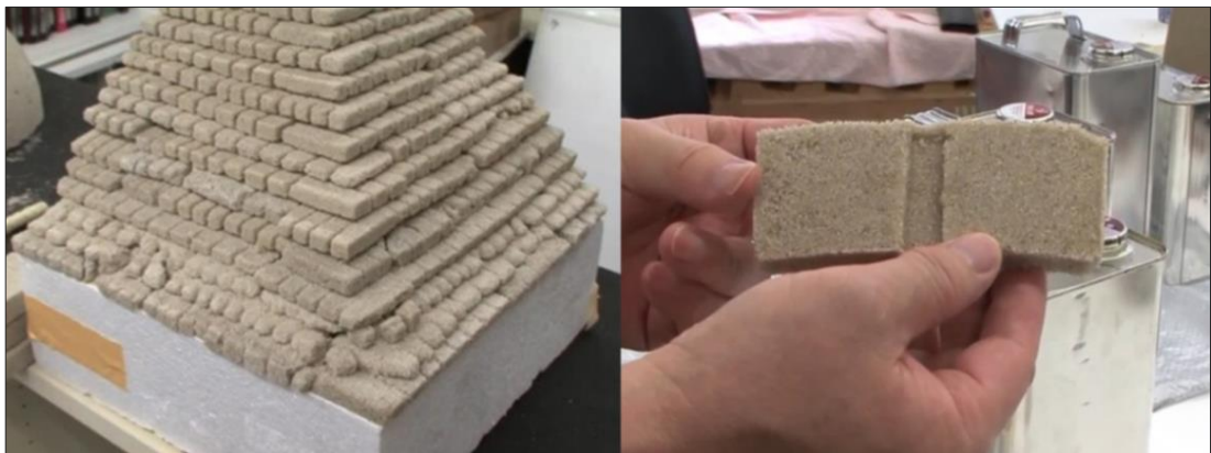
Figure 3.17: The CO 2 Sand Bricks developed by Tis & Partner Japanese company, (2011), Source: (URL16)
