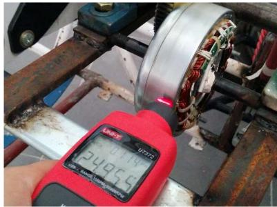
Figure 53: Motor spinning speed measurement setup
