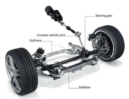
Figure 1: Direct Rack and Pinion steering system [18]
