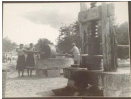
Figure 7. Olive oil production in Çatalköy Olive Oil Mill by using the human/man power, 1938
