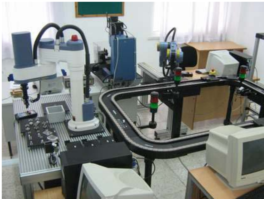
Figure 6-3: Flexible Manufacturing System (FMS) Laboratory of Eastern Mediterranean University
