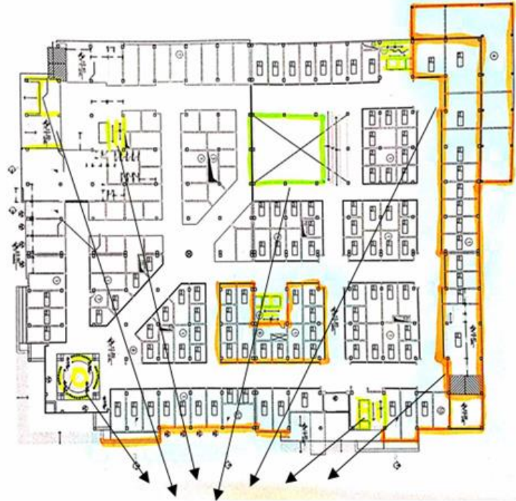
Fall hazardous locations on 2D plan Figure 3: Traditional fall prevention plan
