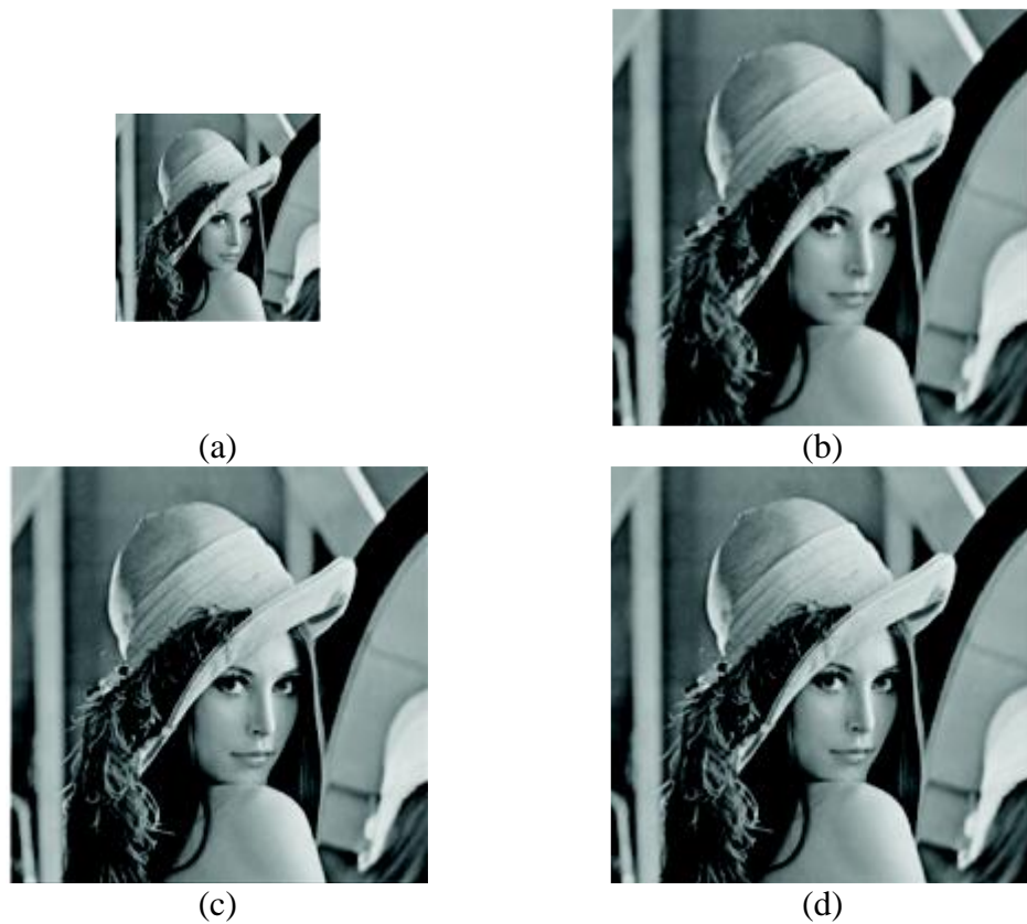
Figure 5.5: The visual comparison between: (a) original LR Lena image and the super resolved image by using (b) Bicubic interpolation, (c) Irani and Peleg SR technique, and (d) the IIBP method
