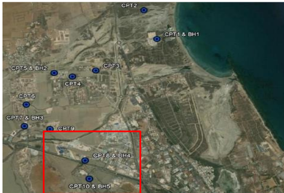
Figure 3.24: Cone penetration tests and borehole locations for Tuzla region (Erhan, 2009 (scale 1:500))
