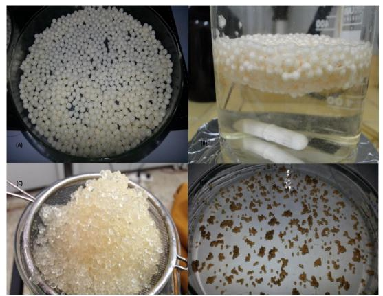
Figure 5.(A)Chitin beads with CaCO<sub>3</sub> (B) Chitin beads in 3M HCl, (C) Porous Chitin Beads before dry, (D) Porous Chitin Beads after drying
