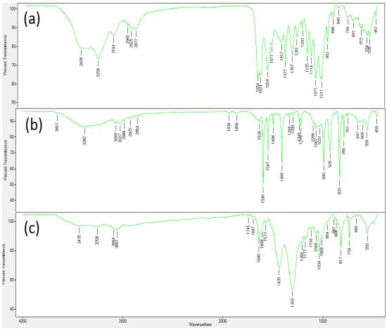
Figure 6. FTIR Spectrum of (a) Chitin, (b) (4VP) and (c) Chitin-*graft*-P4VP Respectively.
