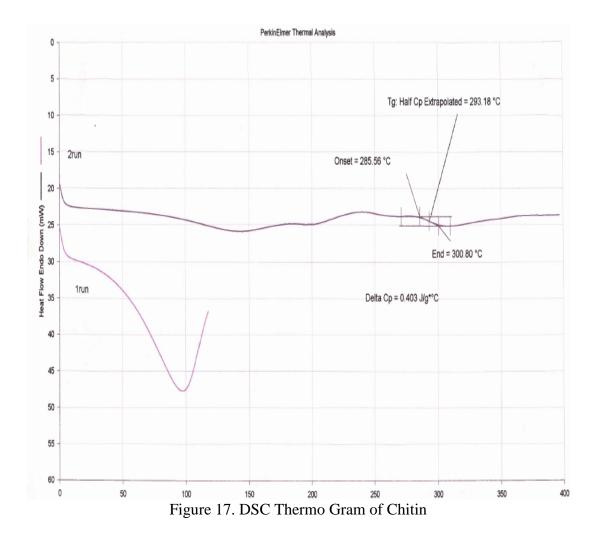
In the first run carried out up to 120 °C, water loss at 90 °C is observed. In the second run studied up to 400 °C, the glass transition temperature of chitin is observed at 293 °C. In the DSC thermo gram of chitin-*graft*-P4VP, two exothermic decomposition peaks are observed at 164 °C and 174 °C. Hence, thermal stability of chitin has been decreased significantly up on grafting with P4VP.
