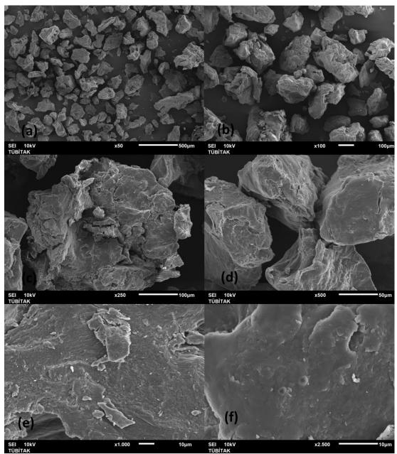
Figure 14. SEM Micrograph of the Chitin, (a) is X 50, (b) is X 100, (c) is X 250, (d) is X 500, (e) is X 1000, (f) is X 2500
