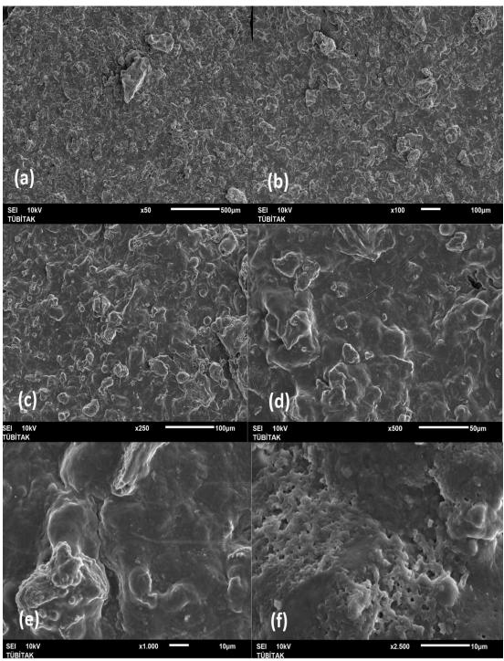
Figure 16. SEM Micrograph of the Grafted Chitin-*graft*-P4VP (380%), (a) is X 50, (b) is X 100, (c) is X 250, (d) is X 500, (e) is X 1000, (f) is X 2500
