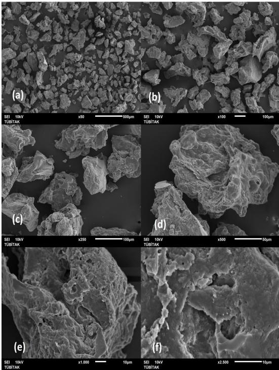
Figure 15. SEM Micrograph of the Grafted Chitin-*graft*-P4VP (48%), (a) is X 50, (b) is X 100, (c) is X 250, (d) is X 500, (e) is X 1000, (f) is X 2500
