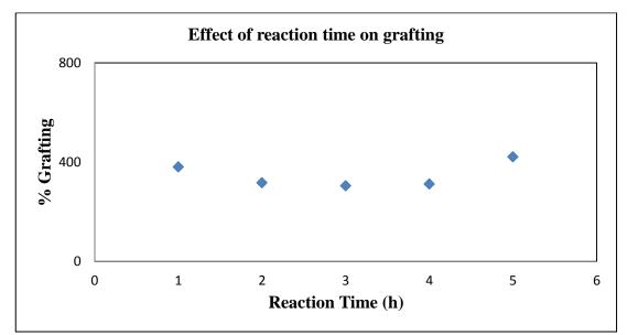
Figure 13. Effect of Reaction Time on Grafting
