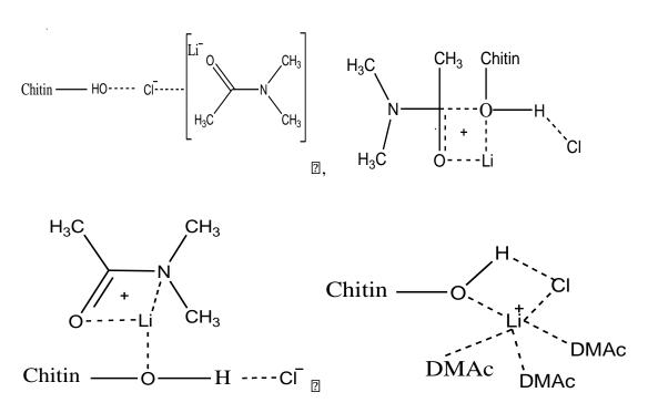
Figure 2. Some Suggested Structures for the Dissolution of Chitin in DMAc-LiCl Solvent System (Oylum, H.,2013).
