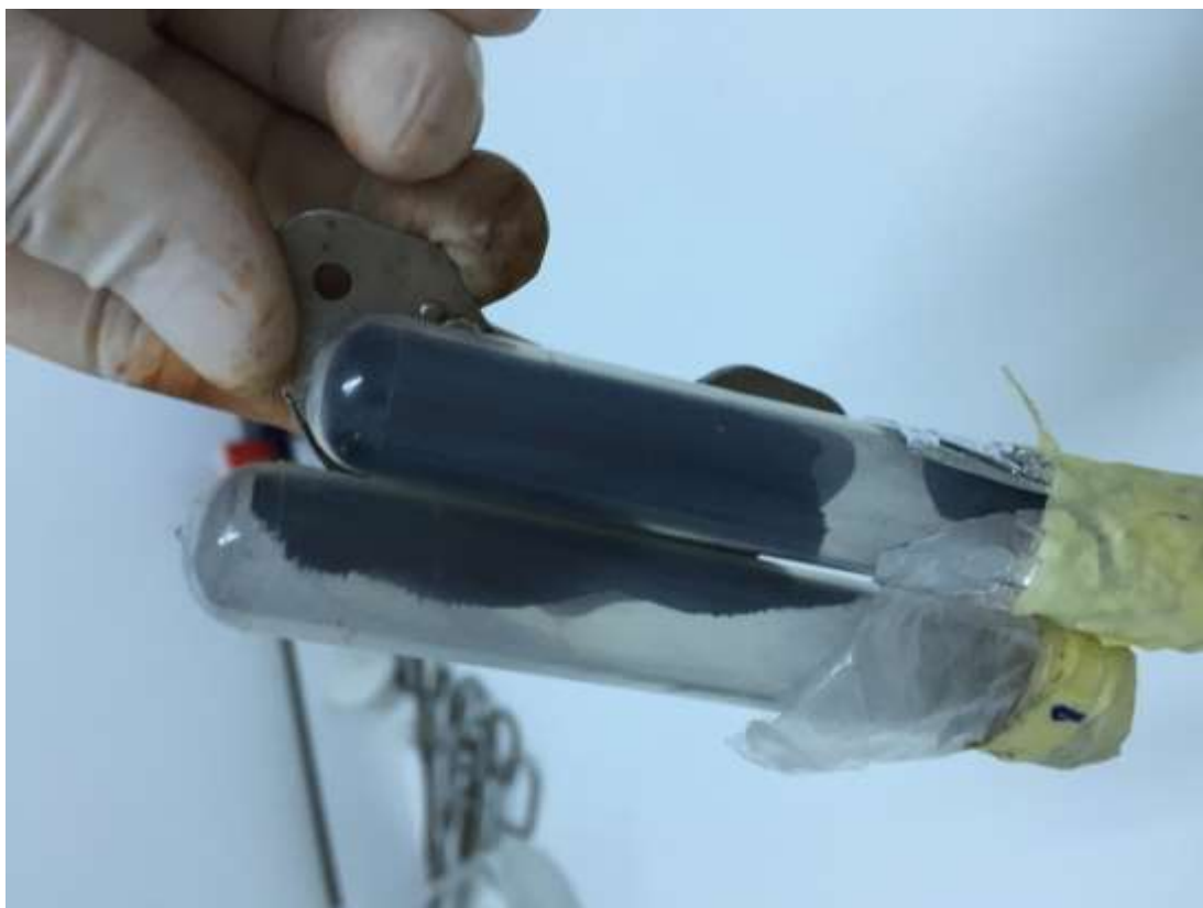
Figure 6: Magnetic biochar derived from palm seeds (adsorbent) (taken by Kola)
