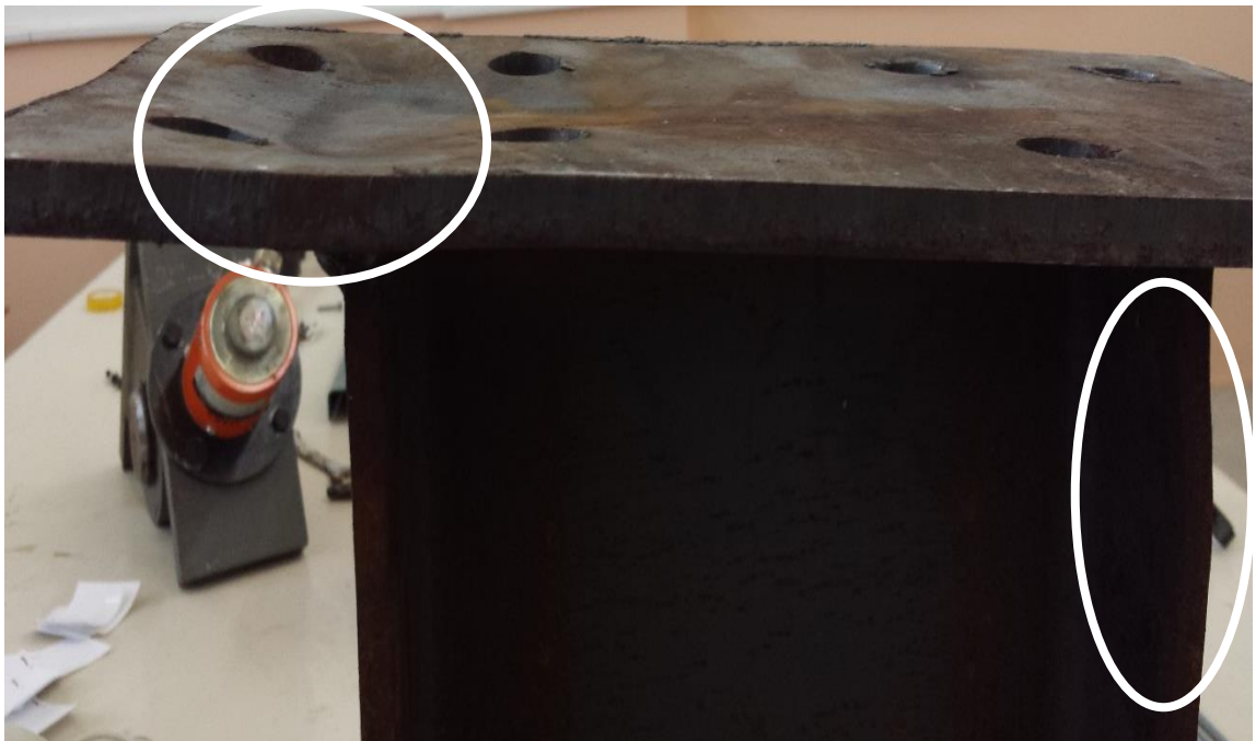
Figure 4.1. Test F200x300 failure mode
