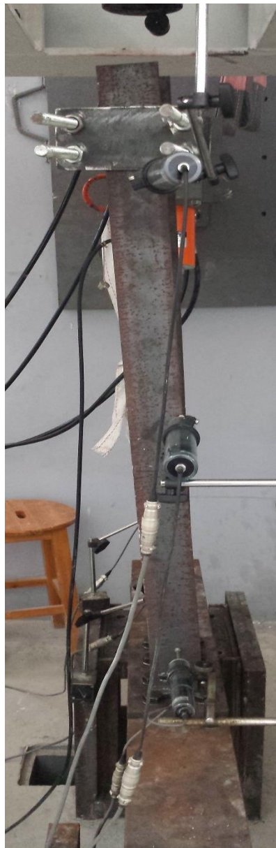
Figure 4.10. Test F160x160 failure modes
