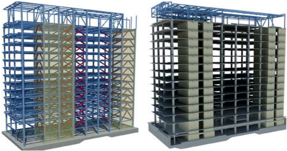
Figure 2.2. Braced frame and shear wall systems
