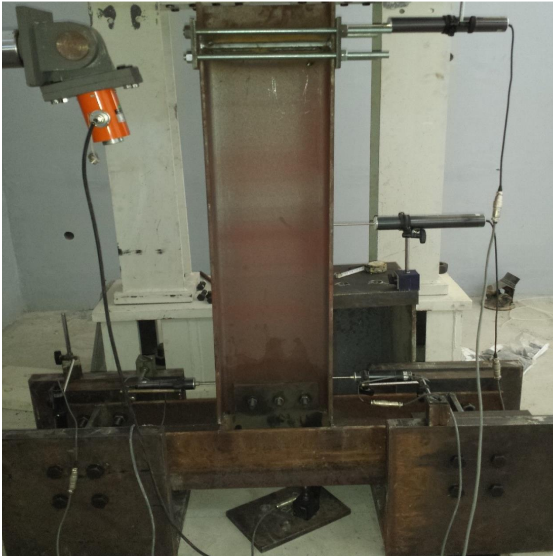
Figure C.1. F200x300 connection Setup
