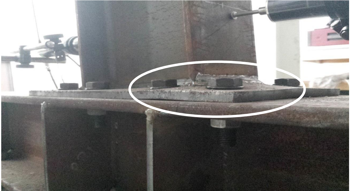
Figure 4.5. F200x200 connection deformation
