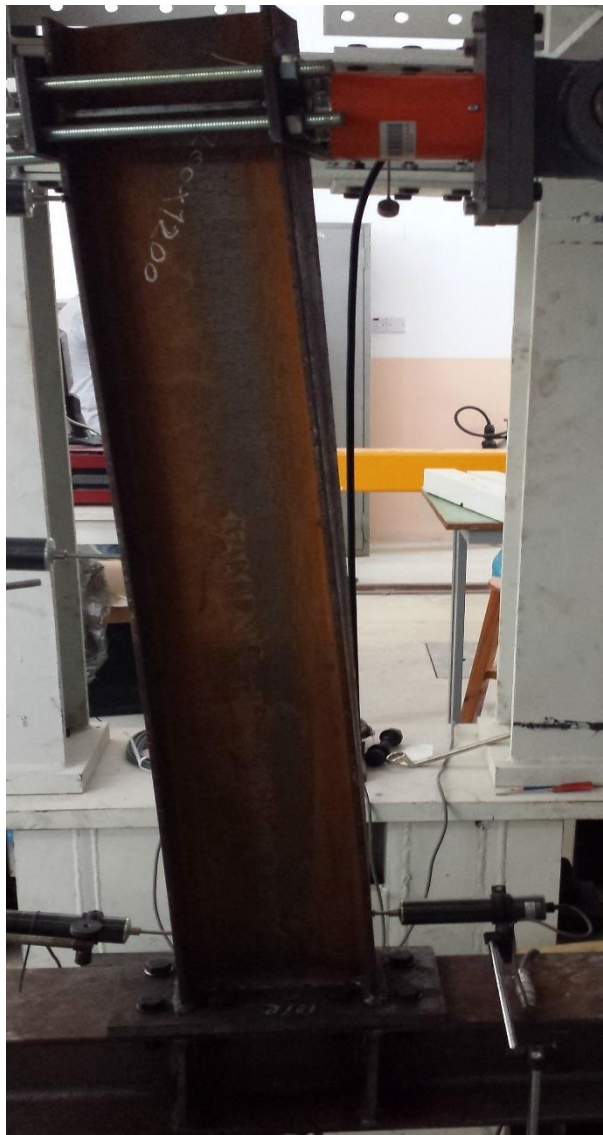
Figure 4.7. Test F160x200 failure mode
