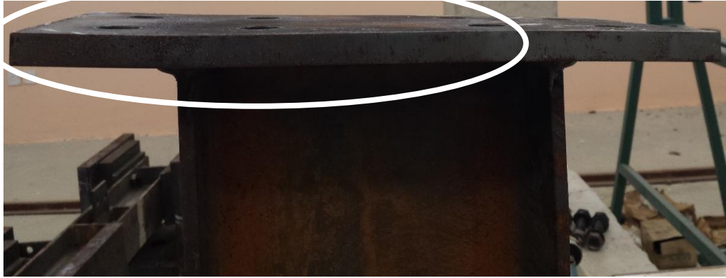
Figure 4.11. F160x160 connection deformation
