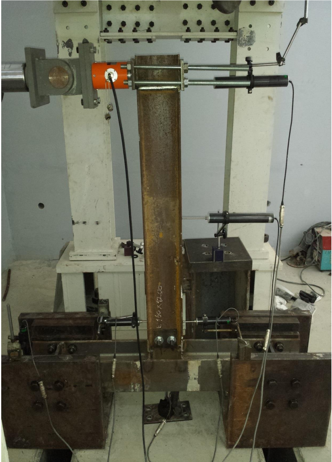
Figure C.28. W16x160 connection setup
