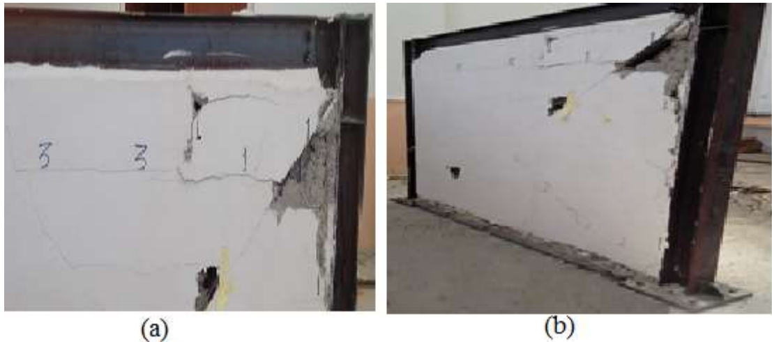
Figure 4.18: Failure modes, (a) corner crushing due to compression (b) horizontal crack along the beam length of test frame MAJ-BFIN8 after testing.
