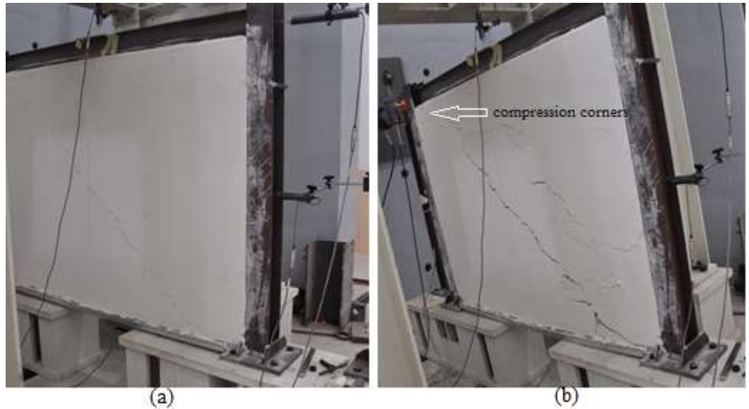
Figure 4.5: Diagonal cracks of the infill wall at the location of a compression diagonal bracing for test frame MIN-MFIN2.
