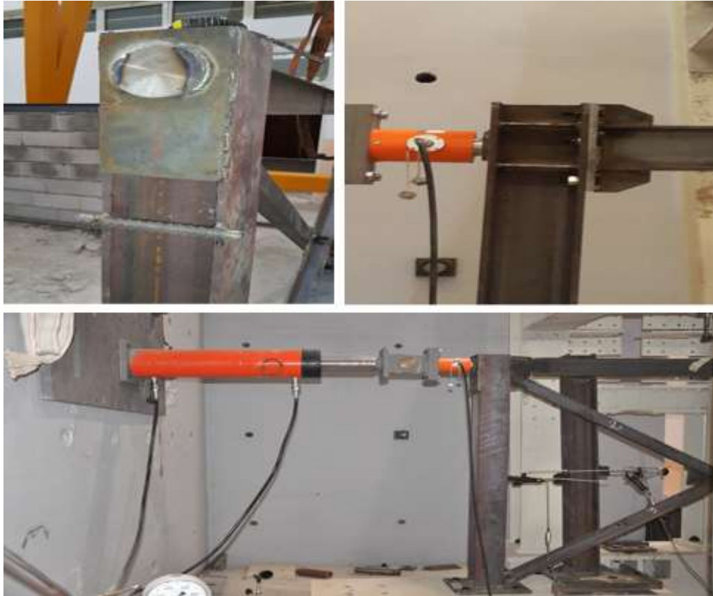
Figure B.9: Set up of hydraulic jack with a capacity of 1000 kN.
