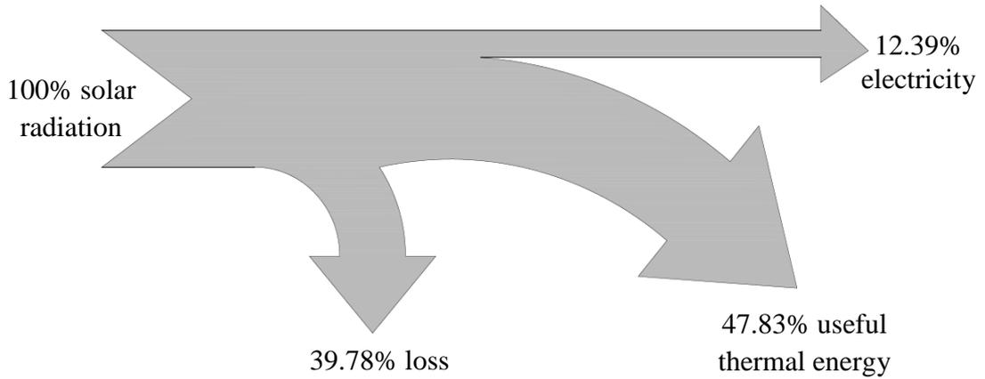
Figure 17. Energy flow diagram of CPV/T collector with two mirrors
