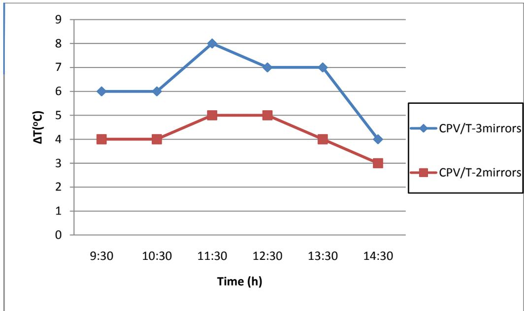
Figure 24. Increment in the temperature of circulated water through the CPV/T collector
