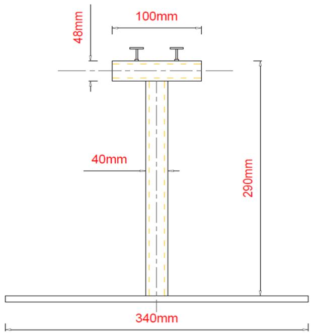
Figure 6. The metal pipe attached on the PV module and the PV/T collector
