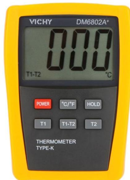
Figure 11. Vichy DM6801A Digital thermometer
