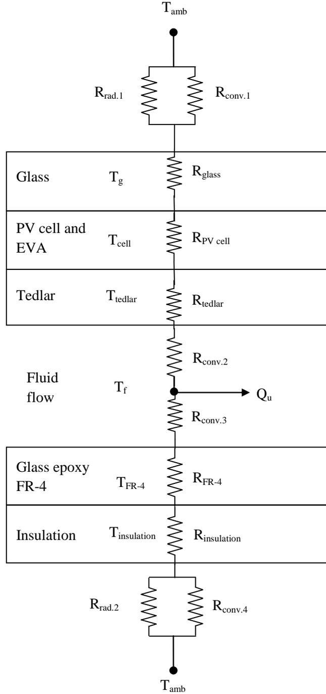
Figure 9. Thermal network of CPV/T collector
