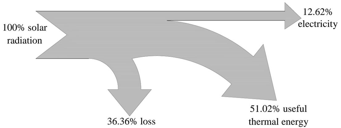
Figure 18. Energy flow diagram of CPV/T collector with three mirrors
