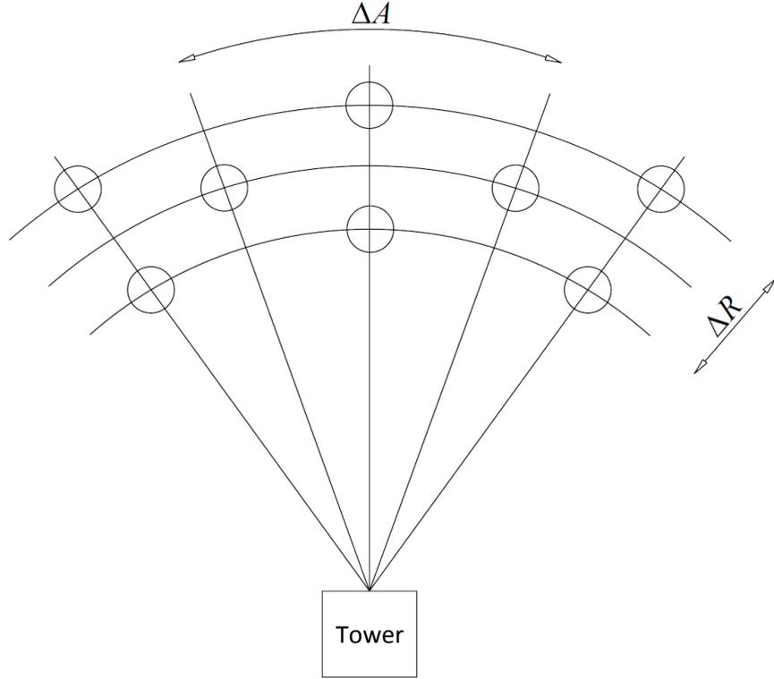
Figure 8. The radial stagger mirror layout pattern
