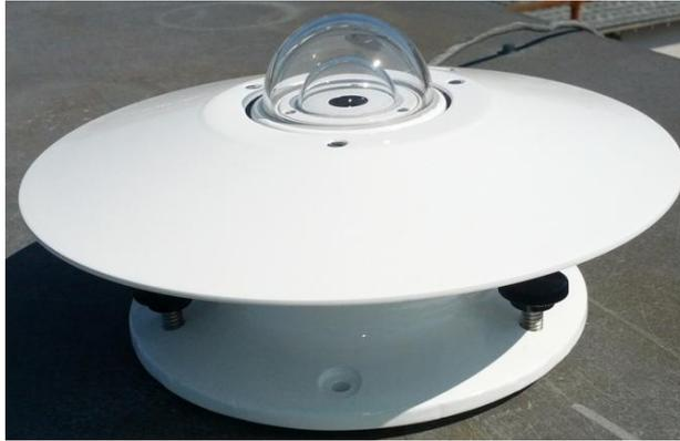
Figure 12. Eppley Radiometer Pyranometer
