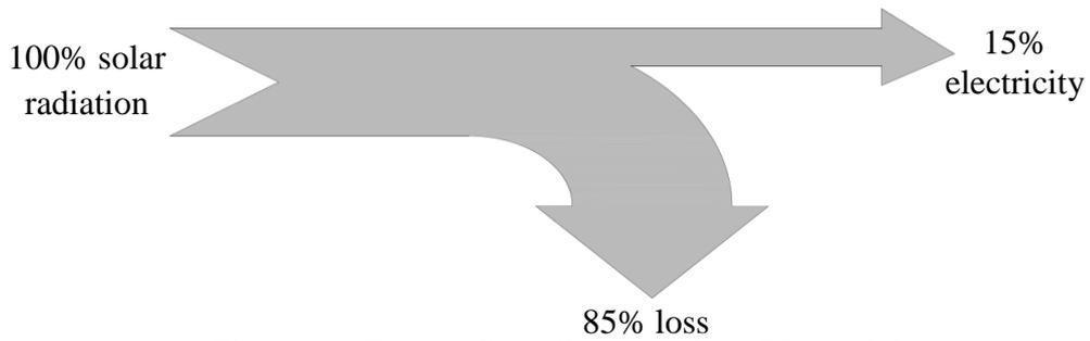
Figure 16. Energy flow diagram of the PV module
