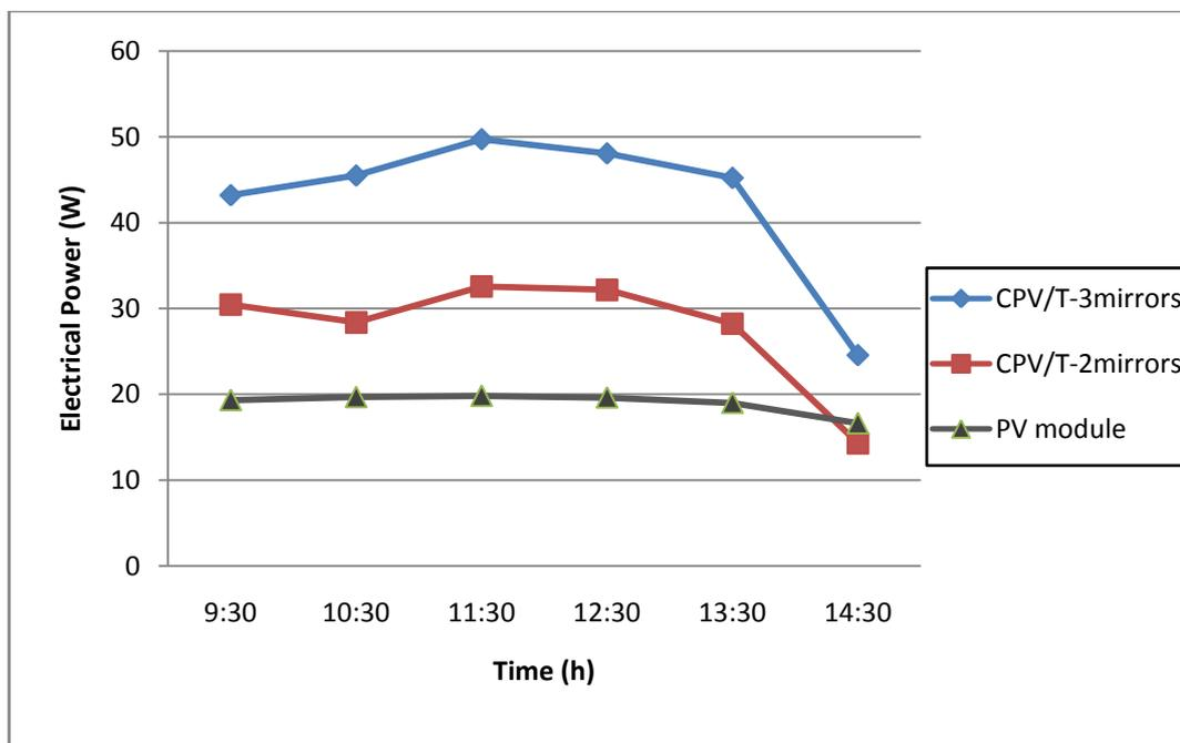
Figure 22. PV module and CPV/T collector electrical power outputs
