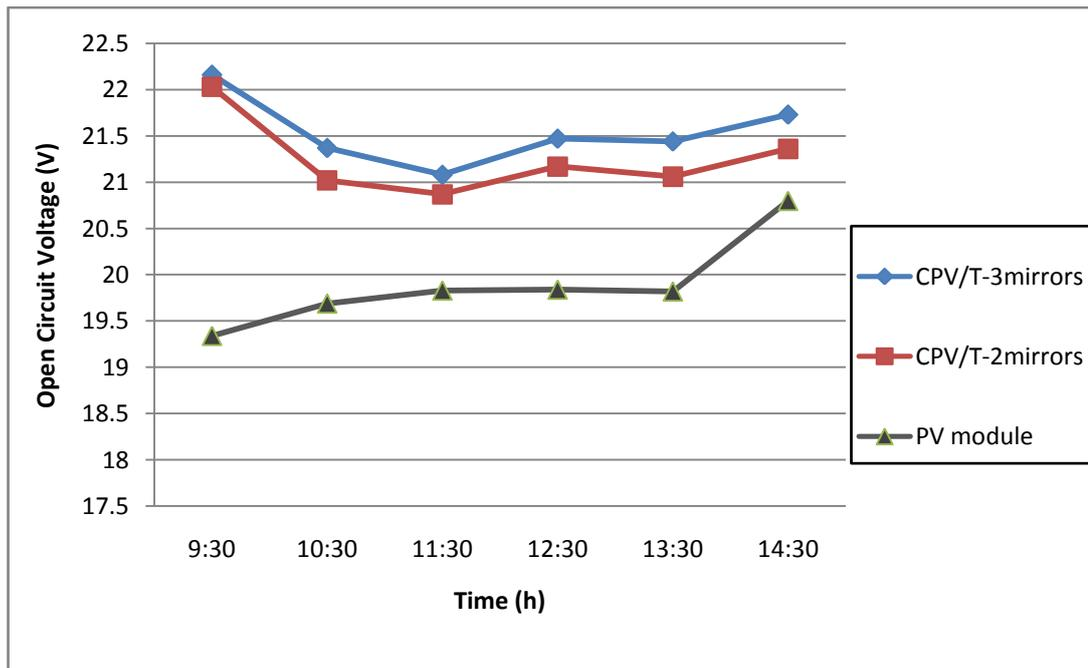
Figure 21. Variation of open circuit voltage versus time during the day of test
