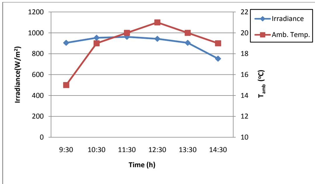
Figure 19. Variation of ambient temperature and solar irradiance during the test day
