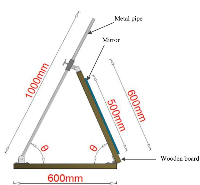
Figure 7. The design of reflectors used in the experiment
