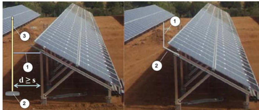
Figure 23: Isolated (left) and non-isolated (right) LPS (Charalambous et al., 2013)
