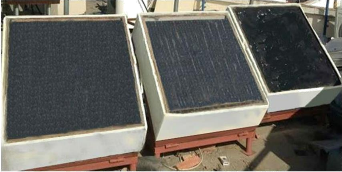
Figure 14: DPGSAHPB with mesh layers, DPGSAHPB with iron wools and transpired SAH
