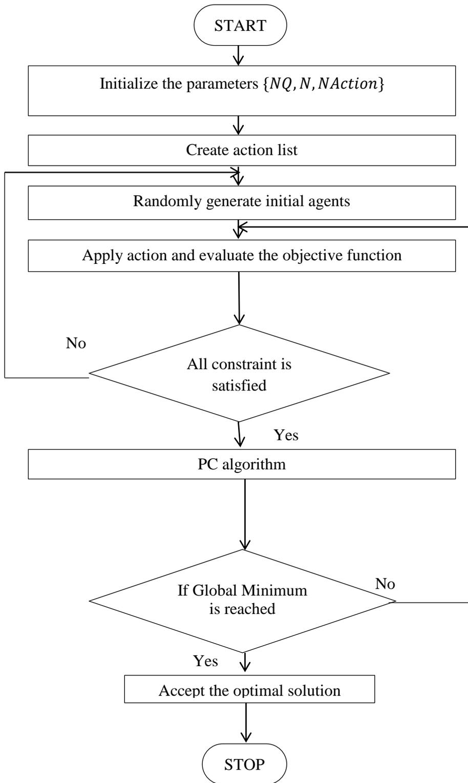
Figure 4.2: Flowchart PC Algorithm for N-queens Problem
