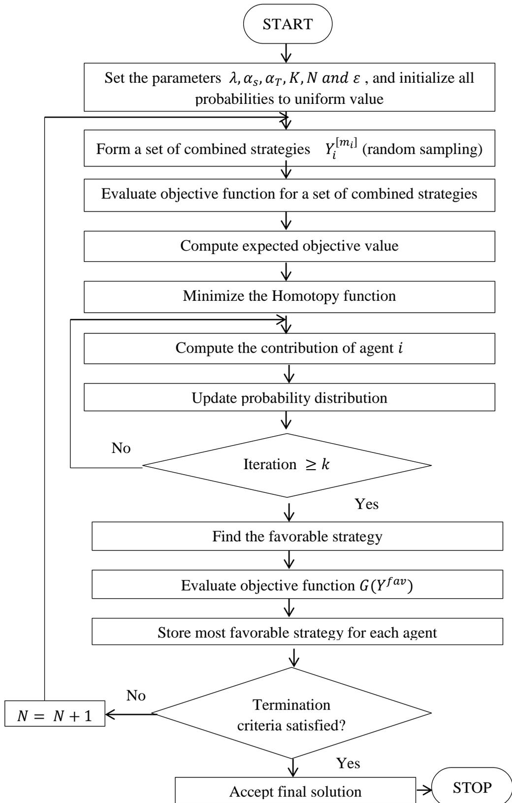
Figure 3.3: Flowchart of PC Algorithm
